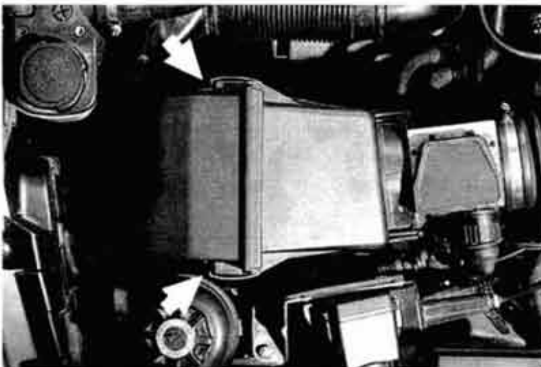
Fig. 5. Air filter housing in front left (driver's) side of M50 engine compartment. Unclip spring clips (arrows) to remove air filter.
