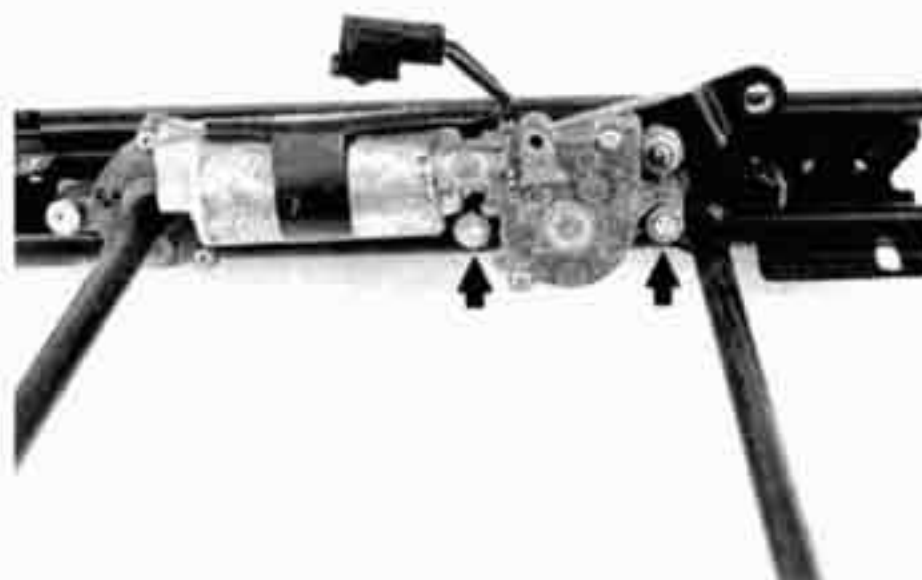
Fig. 10. Seat forward/back motor mounting bolts (arrows).
