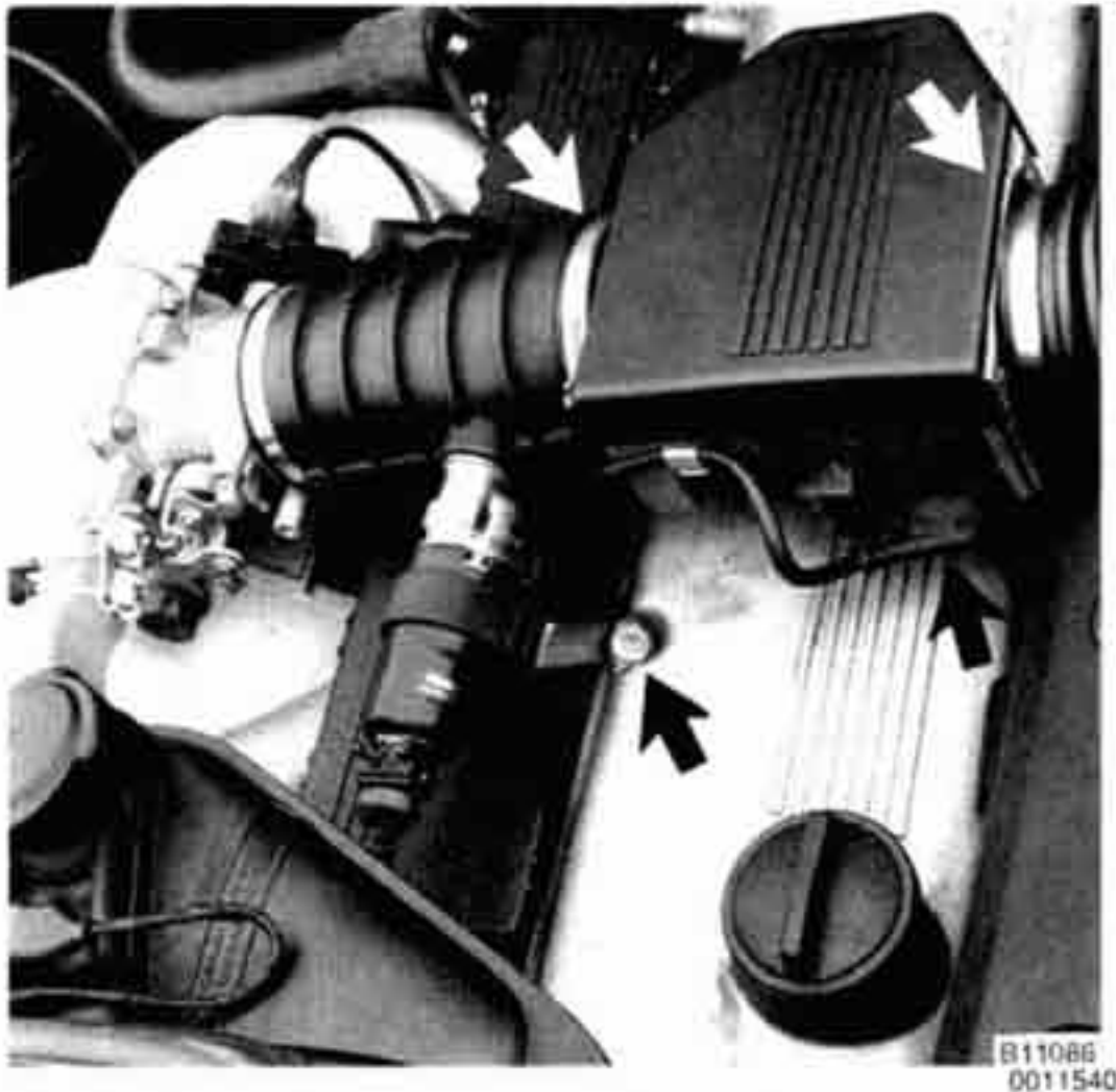
Fig. 4. Idle air stabilizer valve and bracket, air flow sensor connector, and hose clamps to be removed/disconnected (arrows).
