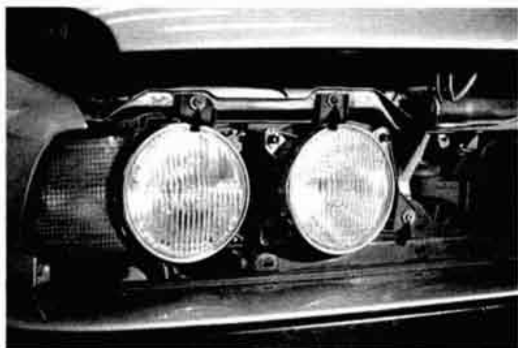
Fig. 3. Headlight assembly front mounting screws (arrows).
