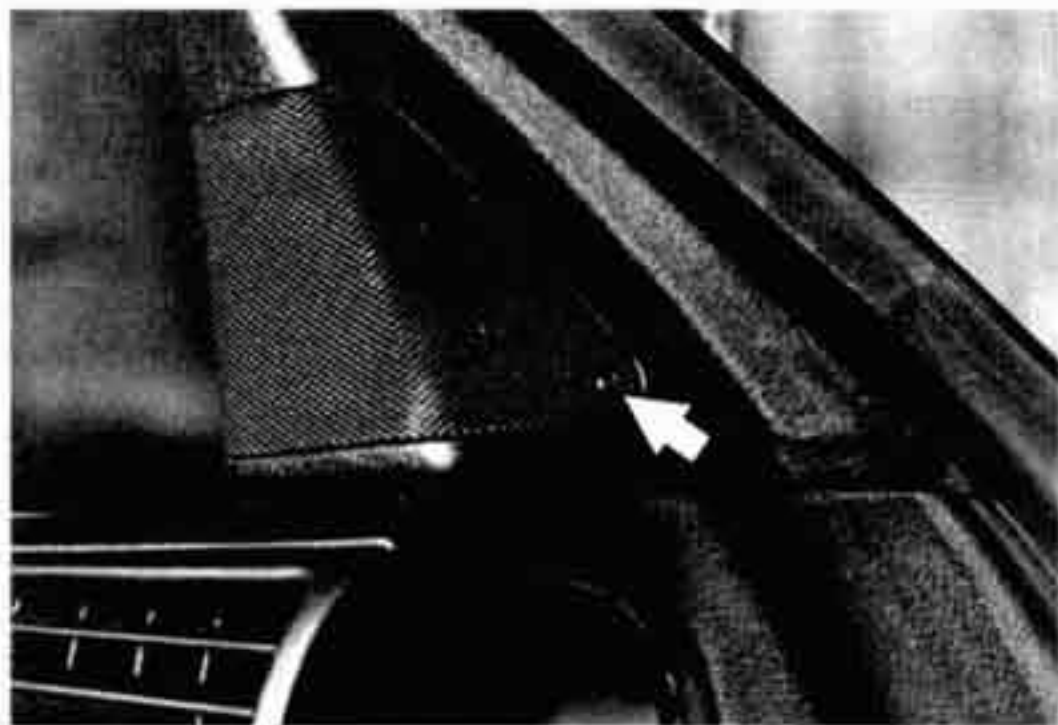
Fig. 3. Door loudspeaker mounting screw (arrow). Pry off plastic cover to access screw.
