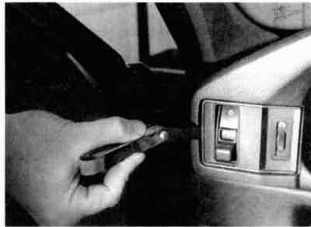
Fig. 6. Feeler gauge being used to release switch frame locking tab.
