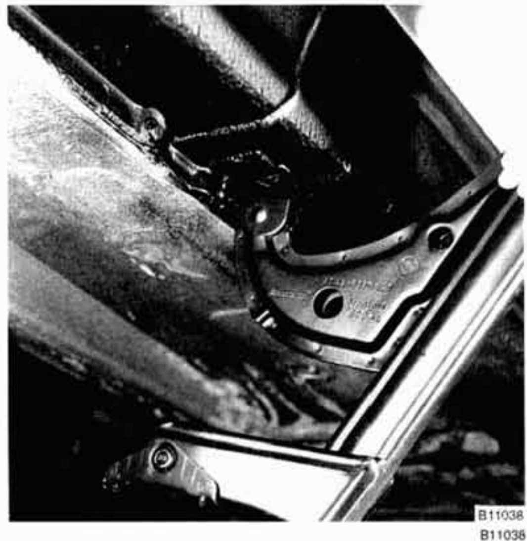
Fig. 2. BMW supplied jack correctly positioned under front jacking point.
