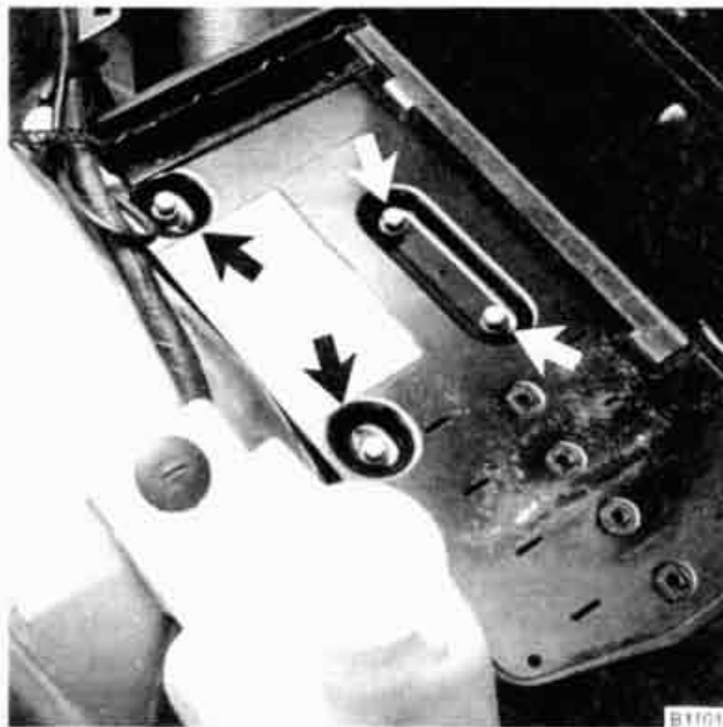
Fig. 9. Battery tray mounting bolts (arrows).
