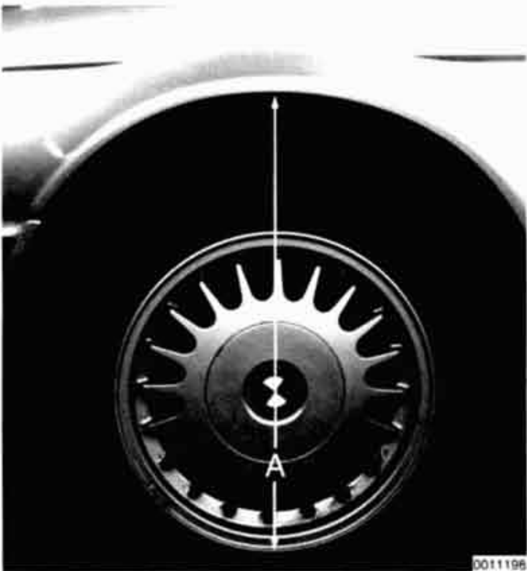
Fig. 2. Ride height measurement (A) is taken from center of wheel arch to bottom of wheel rim. Measure ride height with car in normal loaded position on the ground.
