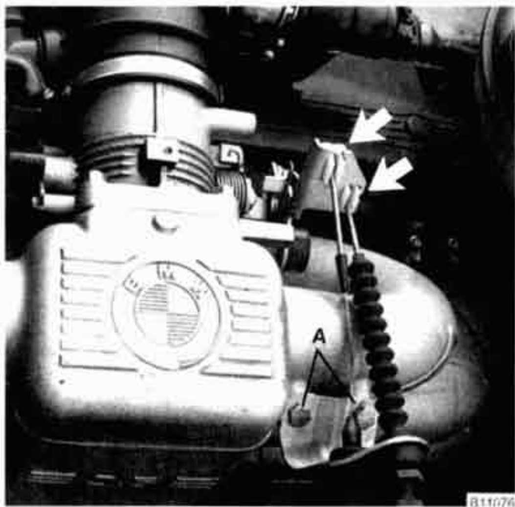
Fig. 36. Disconnect cables at throttle lever (arrows) and remove cable bracket bolts (A).
