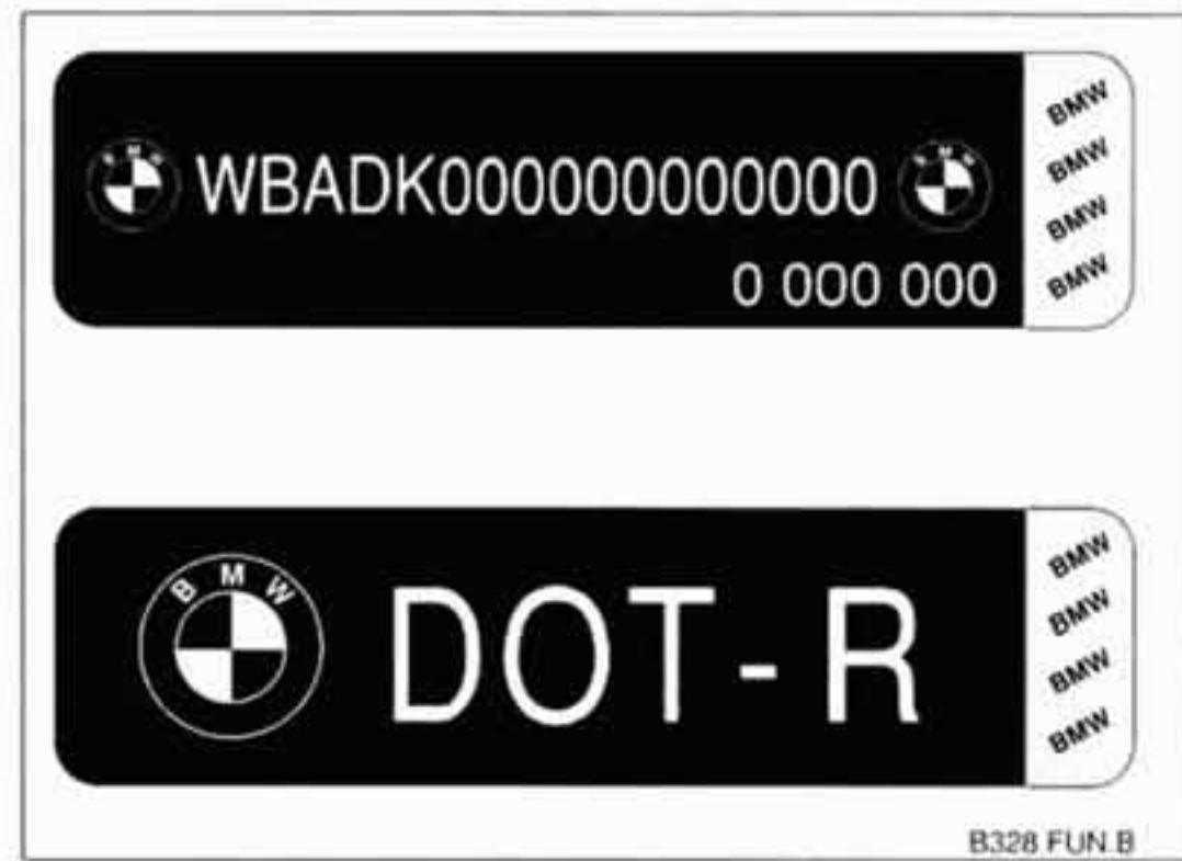
Fig. 6. Labels used to identify parts. Original equipment label with VIN number and roundel logos (top) and replacement part label with one roundel logo.
