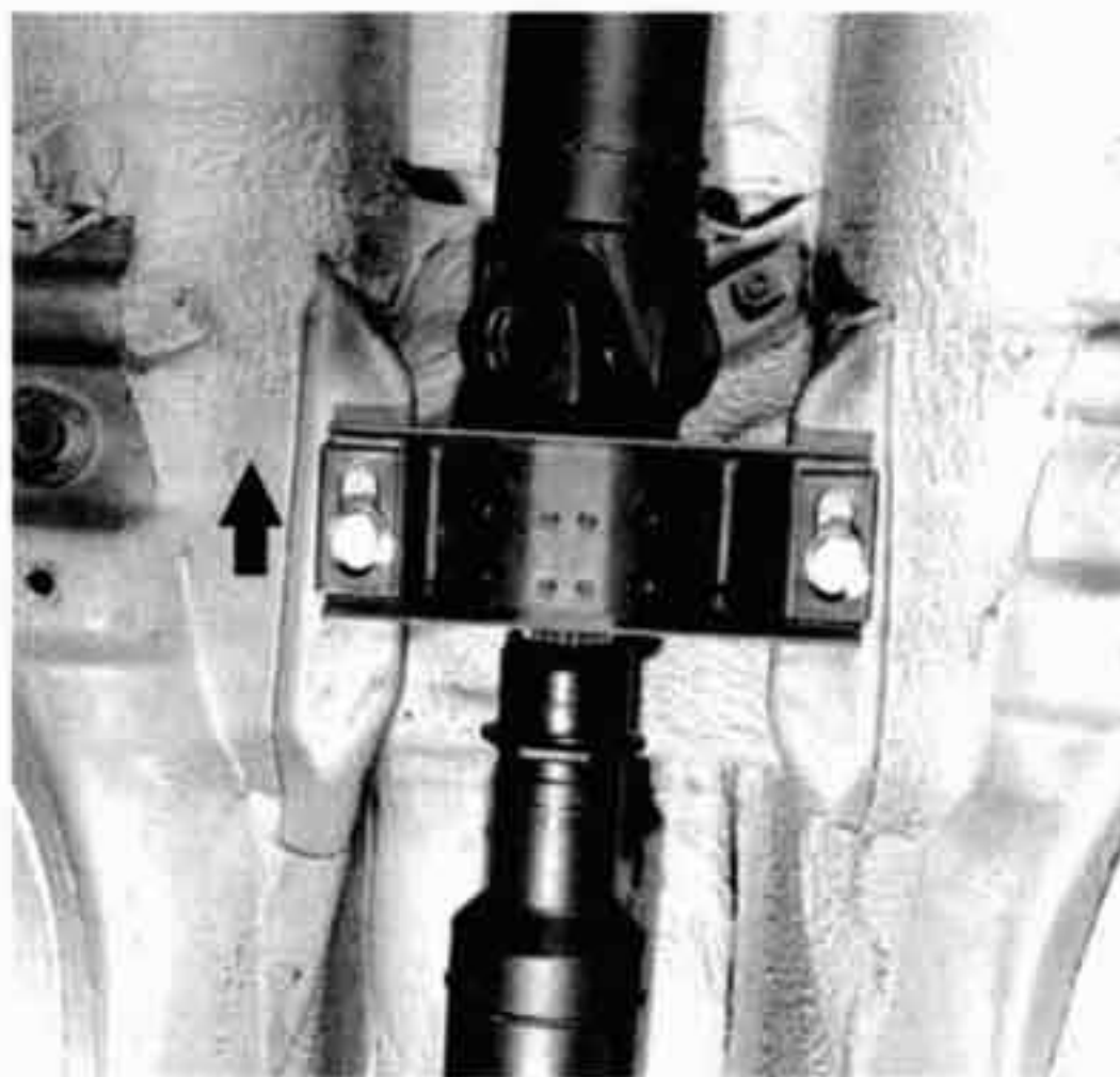
Fig. 8. Preload center bearing toward front 4-6 mm (arrow).
