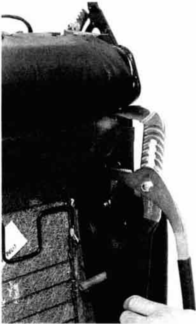
Fig. 11. Release seat back locking lever using pliers.
