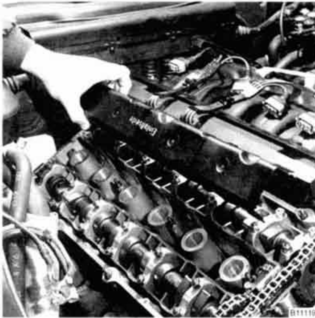
Fig. 5. Oil baffle cover being removed.
