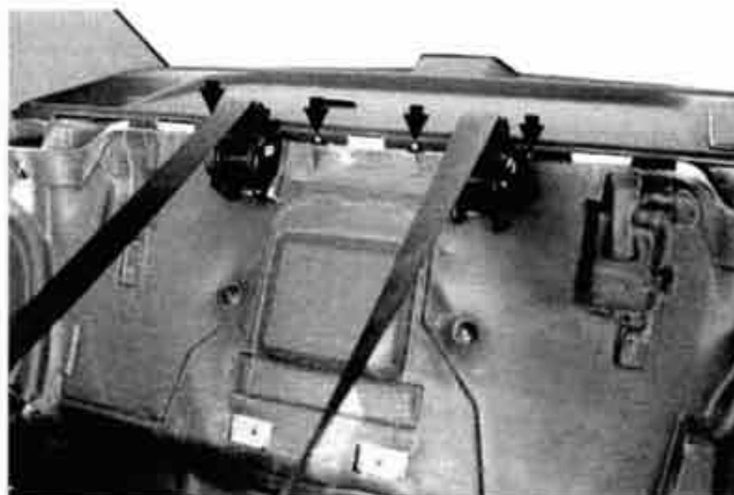
Fig. 5. Parcel shelf retaining clips (arrows).
