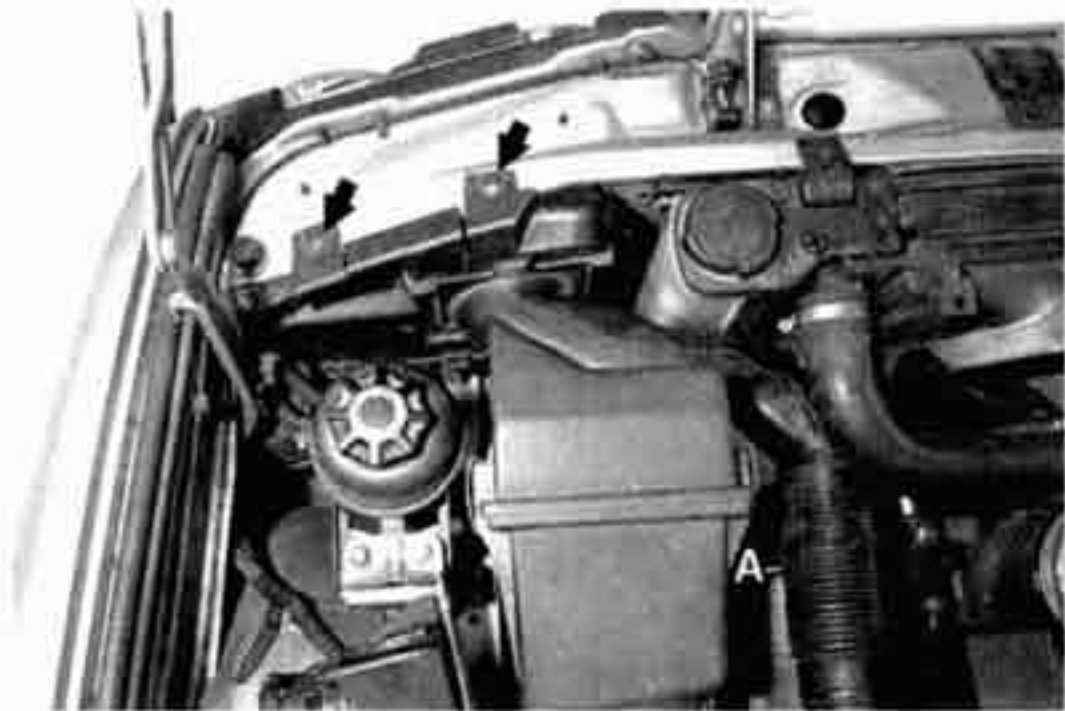
Fig. 1. Headlight protective cover mounting screws (arrows). Alternator cooling duct shown at A.
