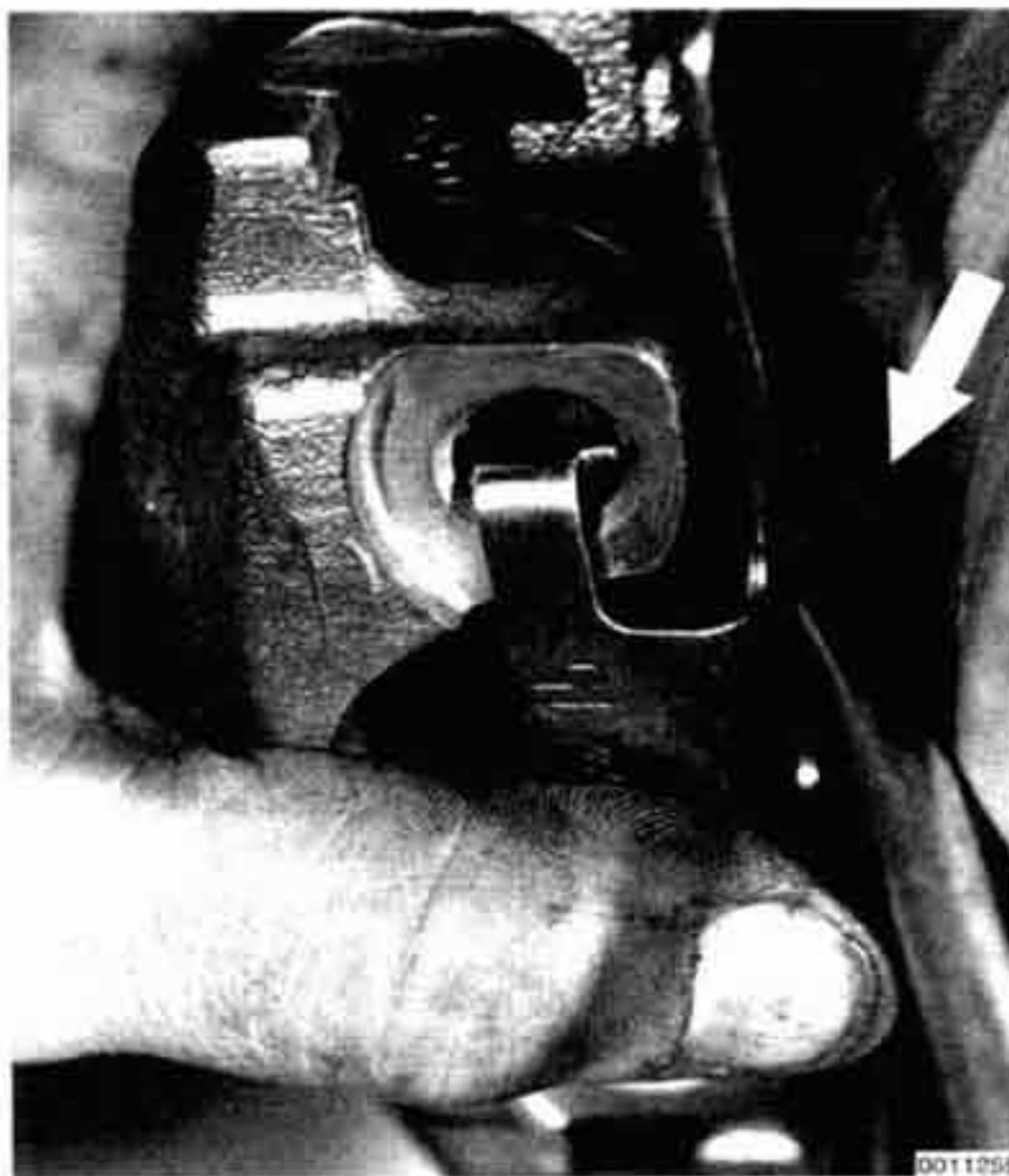
Fig. 3. Brake pad anti-rattle clip being unhooked from caliper using screwdriver (arrow).
