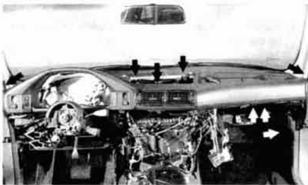
Fig. 7. Instrument panel mounting screws (arrows).
