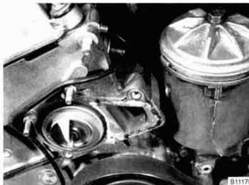
Fig. 16. Thermostat housing shown removed on M50 engine.
