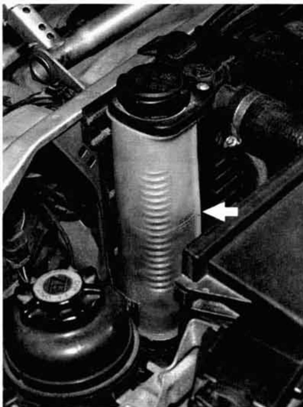
Fig. 13. Fill mark on coolant expansion tank on radiator. Coolant level should be at "cold" mark when engine is cold.
