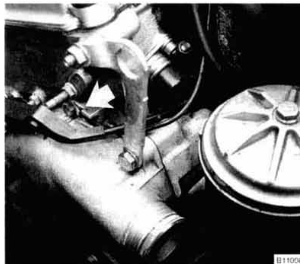
Fig. 10. Main ground (arrow) at front of engine for DME 3.1 and DME 3.3.1. DME 3.1 shown. DME 3.3.1 uses two ground wires at front of engine.
