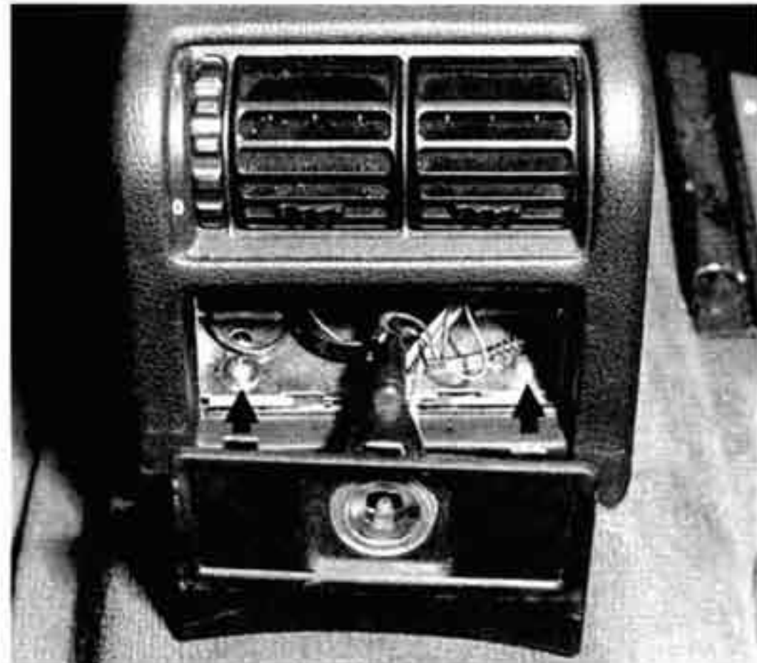
Fig. 1. Center console mounting screws at rear of console (arrows).
