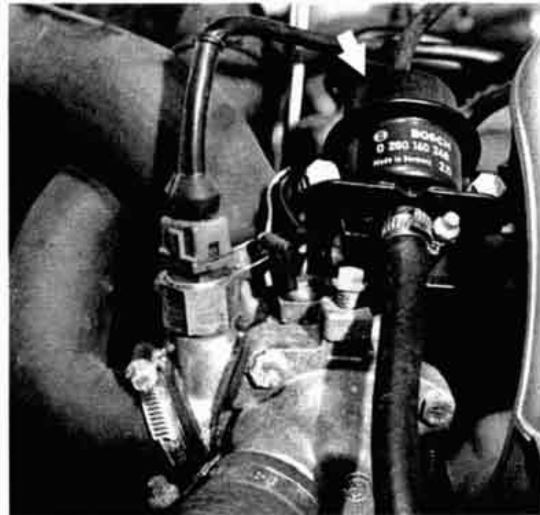
Fig. 24. Fuel pressure regulator (arrow) on M20 engine. M30 engine similar.
