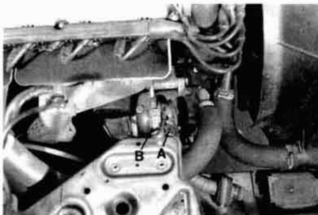
Fig. 18. A/C compressor pressure hose (A) and suction hose (B) on M20 engine.
