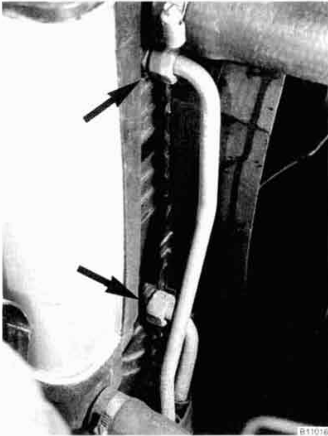
Fig. 10. ATF cooler lines at left side of radiator (arrows).
