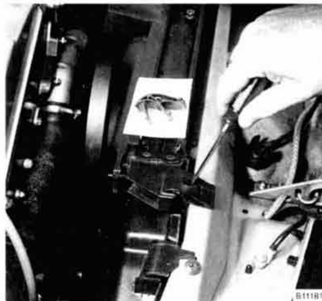
Fig. 19. Radiator retaining clip being removed. Push down and pull screwdriver forward to release clip.
