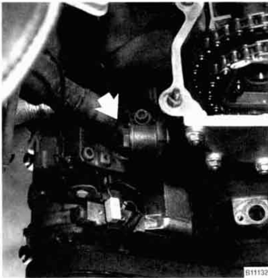
Fig. 17. Primary timing chain tensioner (arrow).
