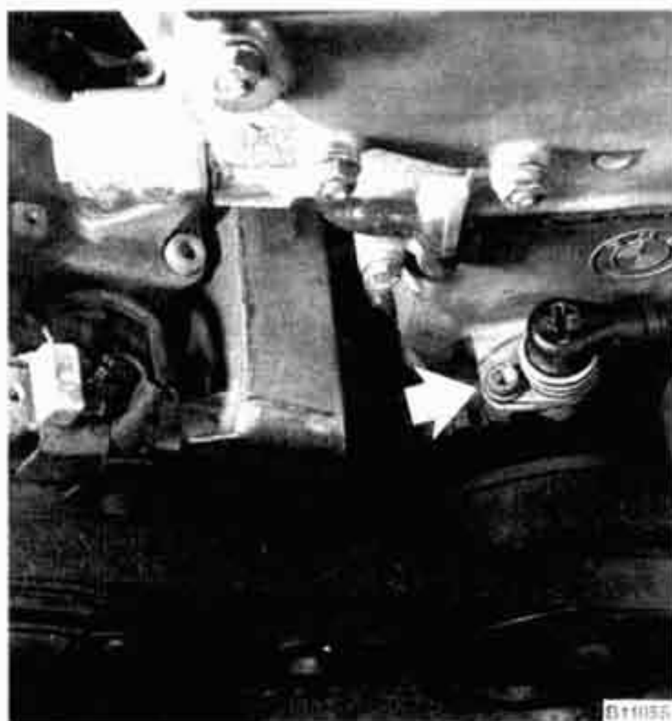
Fig. 17. Reference/speed sensor mounting bolt (arrow).
