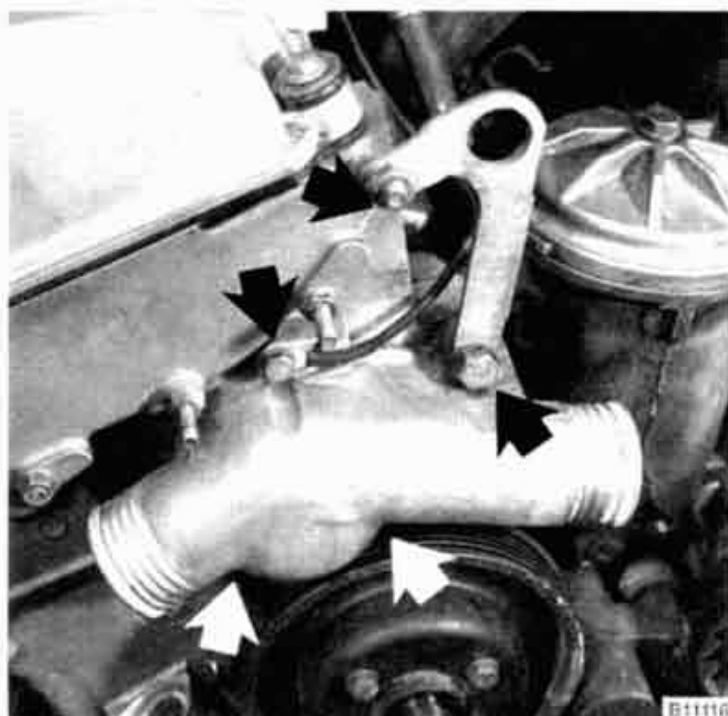
Fig. 2. Engine lifting bracket and thermostat housing mounting bolts (arrows).
