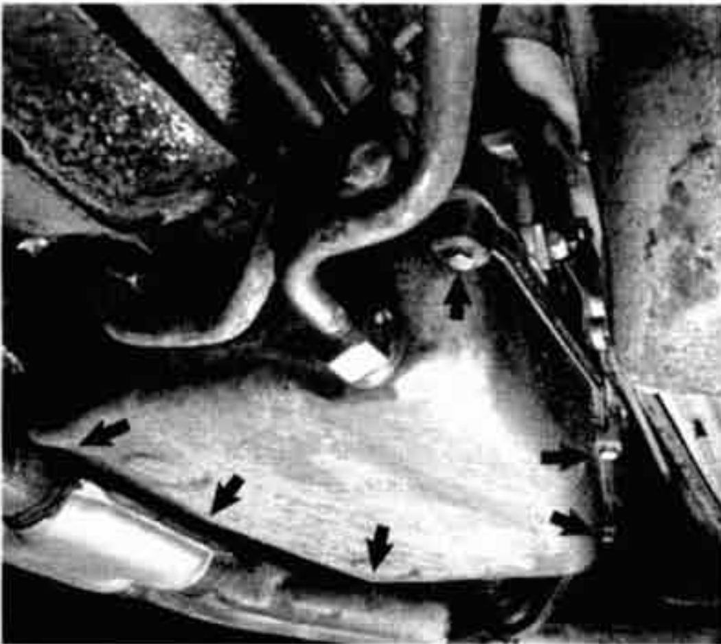
Fig. 22. ATF sump mounting bolts and clamping brackets (arrows).
