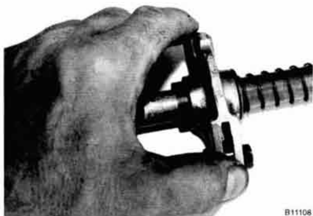
Fig. 38. Rocker arm being checked for wear on rocker arm shaft.
