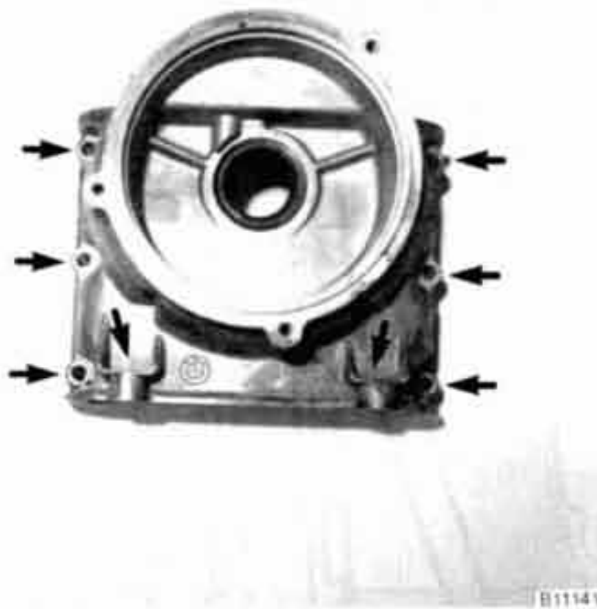
Fig. 24. Upper timing chain cover mounting bolt holes (arrows).
