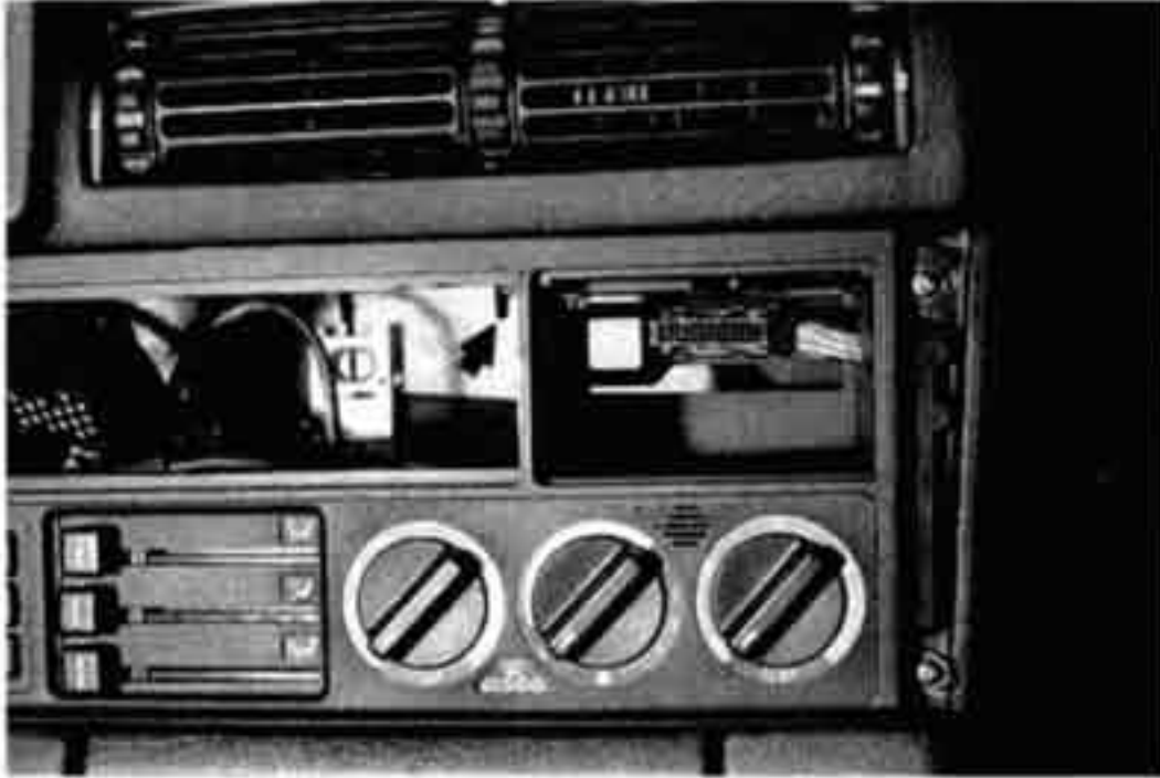
Fig. 11. On Board Computer release lever ( arrow ).
