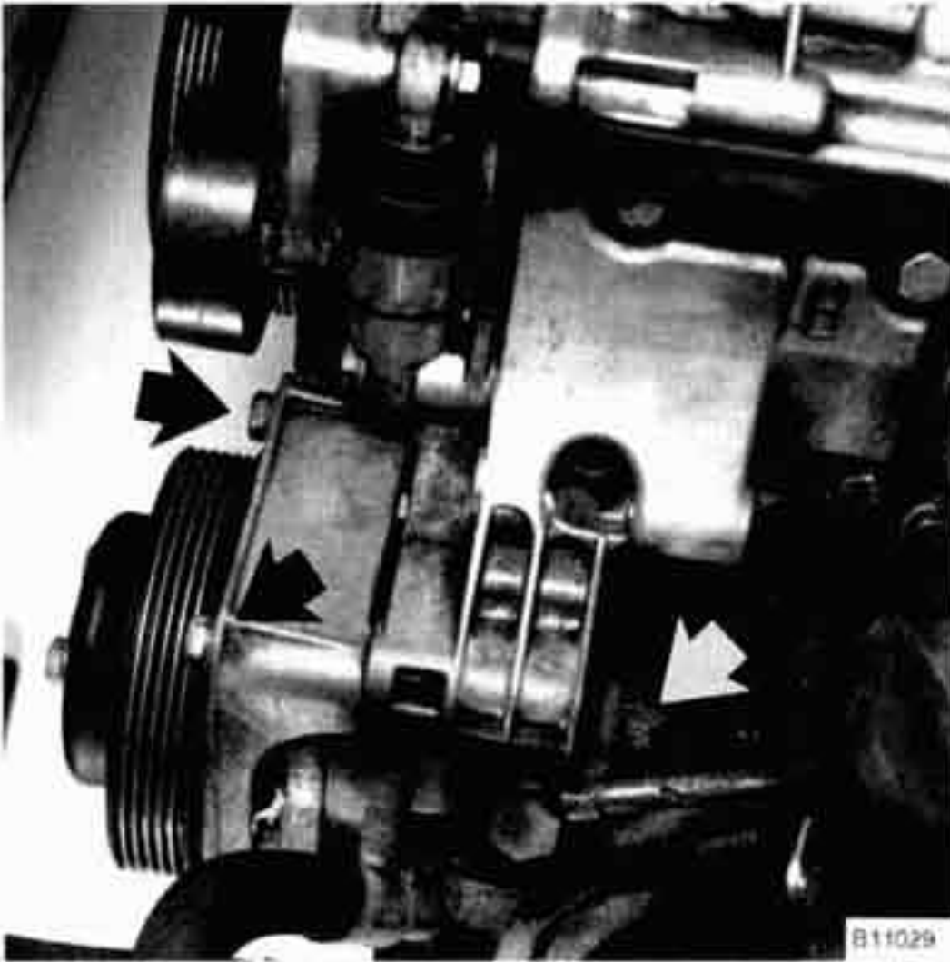
Fig. 23. Power steering pump mounting bolts (arrows).
