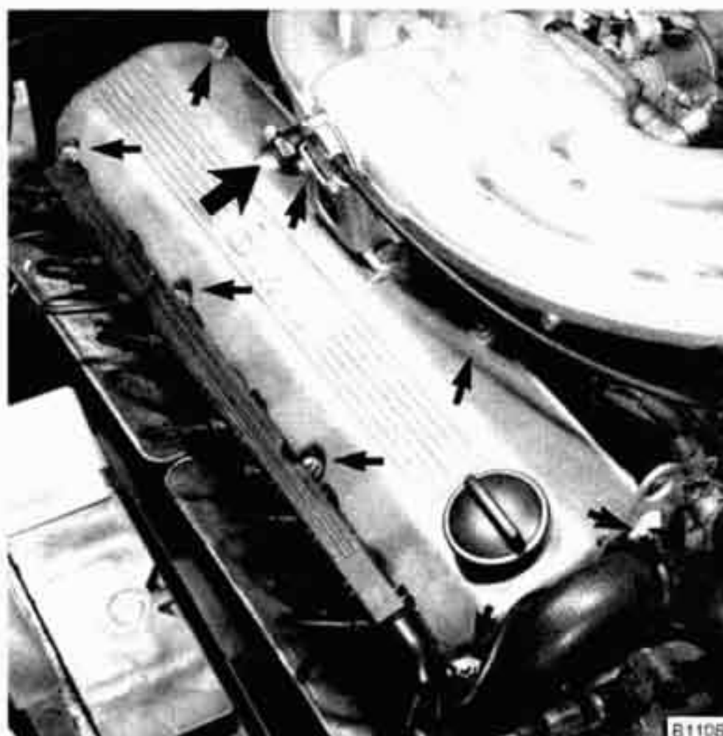
Fig. 2. Breather hose and cylinder head cover mounting nuts (arrows).
