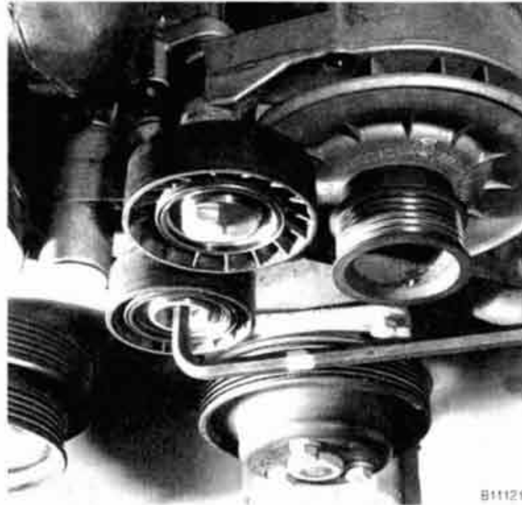
Fig. 7. Drive tensioner roller bolt being removed.
