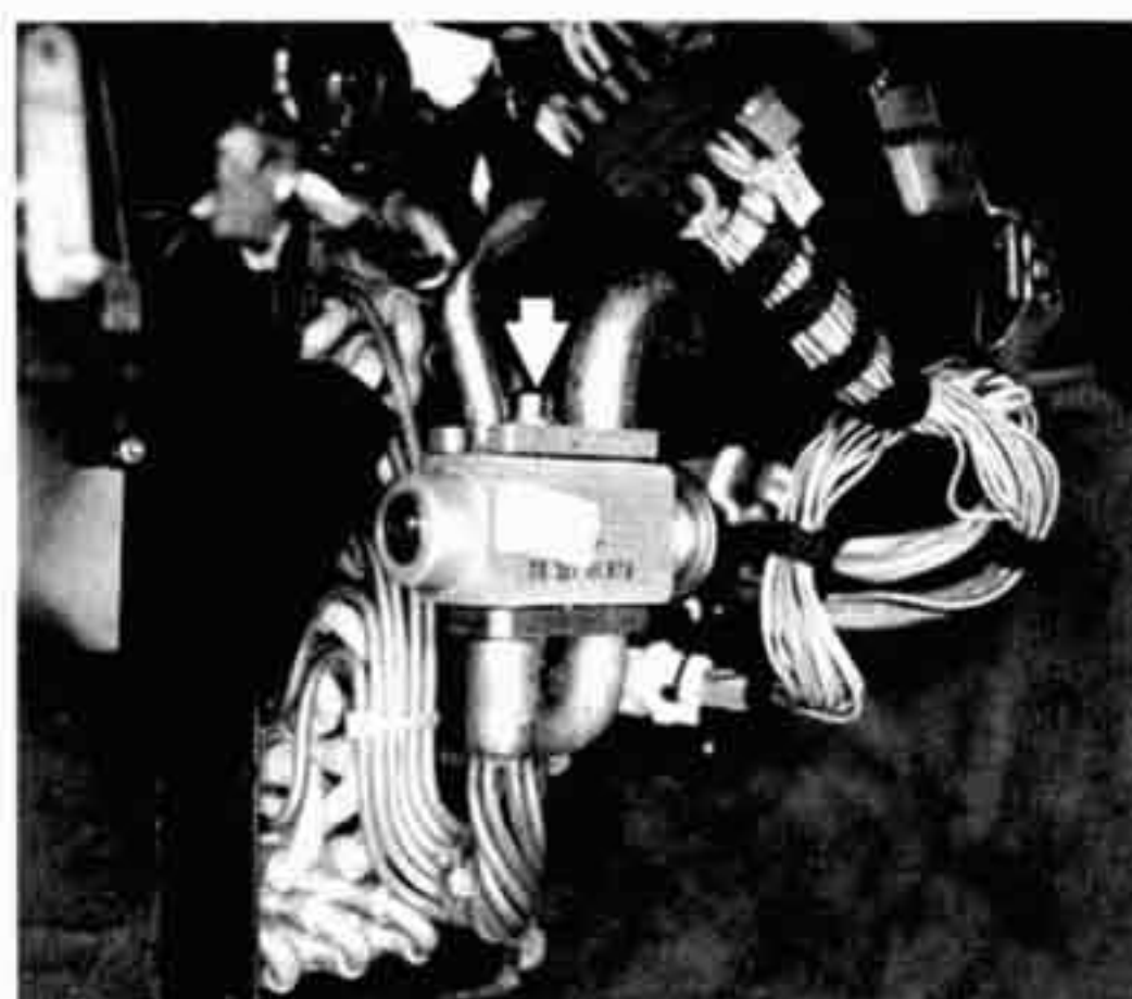
Fig. 27. Refrigerant line fitting mounting bolt at expansion valve (arrow).
