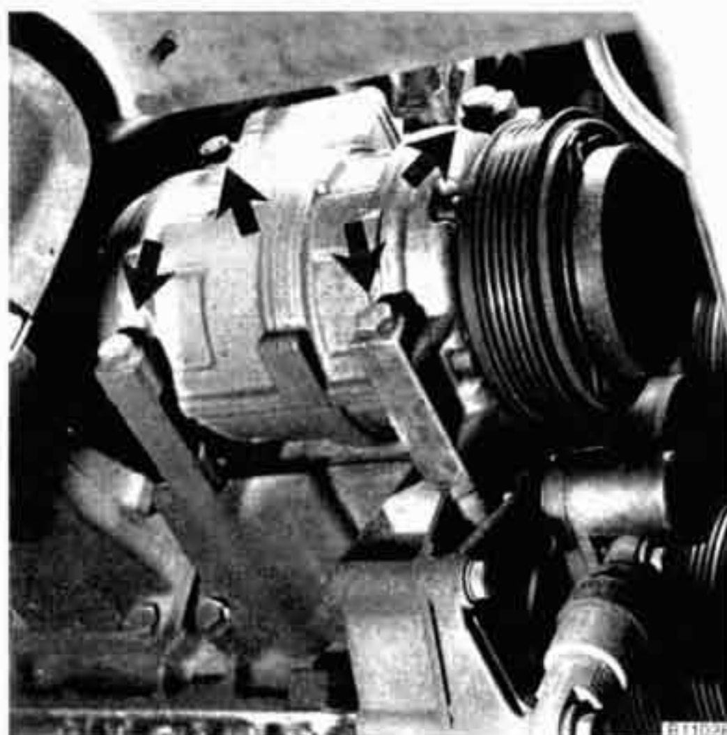
Fig. 22. A/C compressor mounting bolts (arrows).
