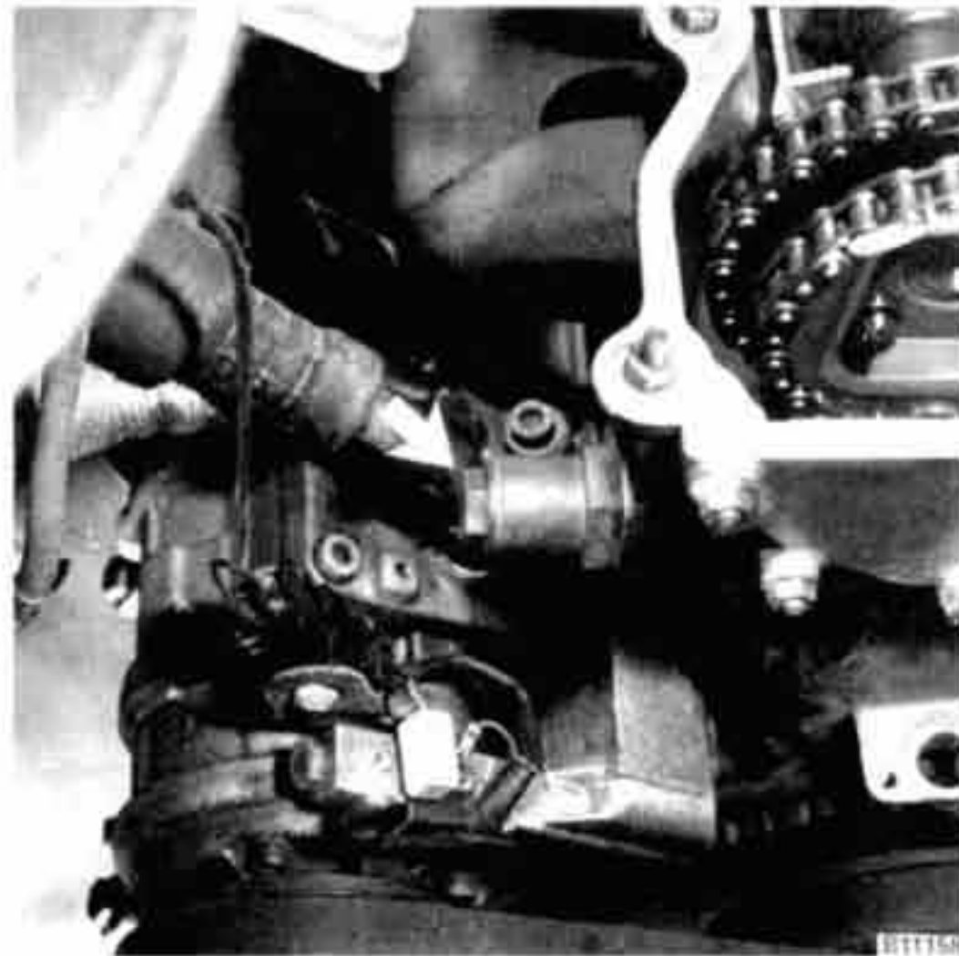
Fig. 40. Primary timing chain tensioner (arrow).
