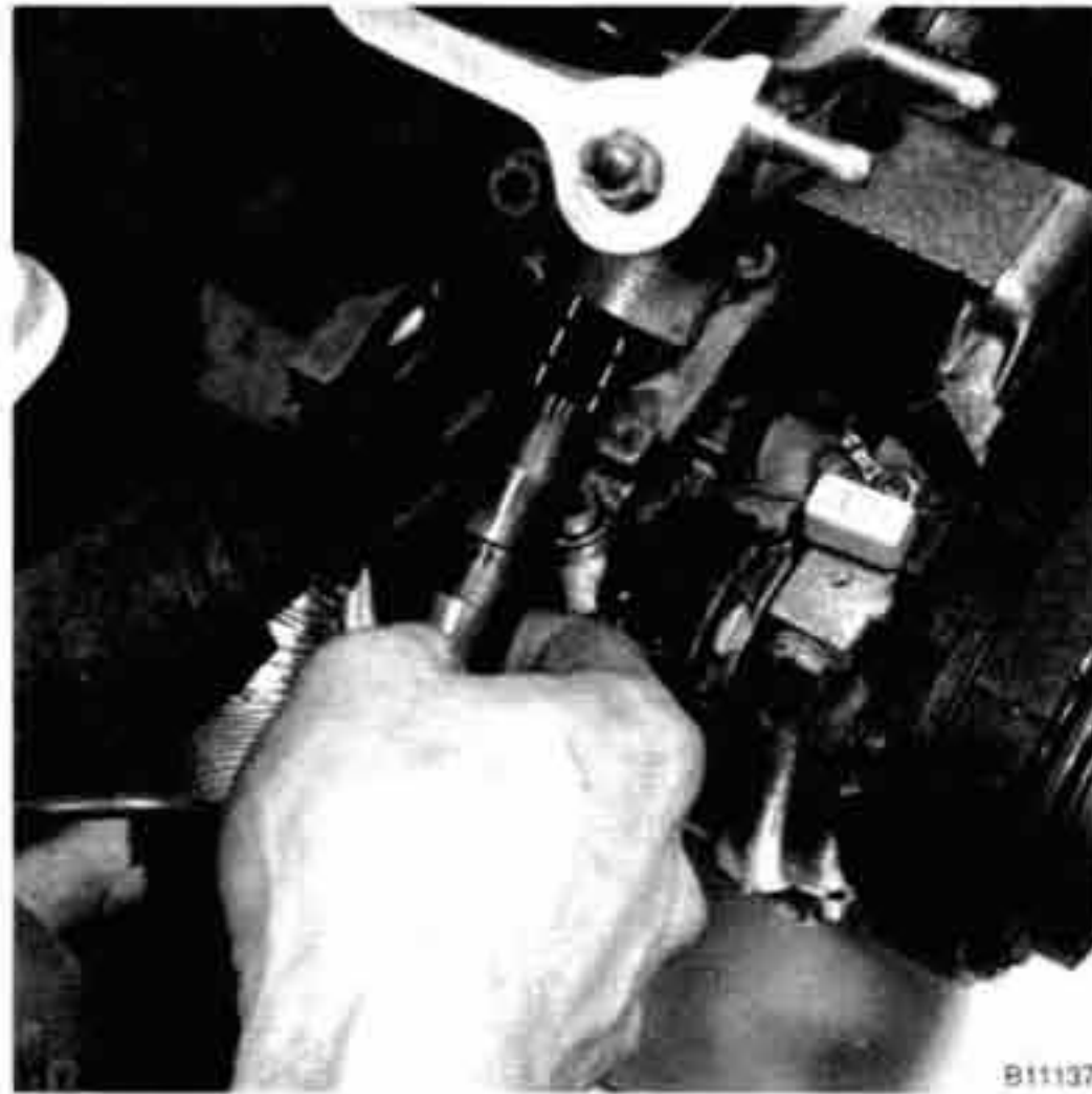
Fig. 21. Primary timing chain tensioner being installed on 1991 and 1992 cars. Piston cutout must be in position shown to engage chain rail.
