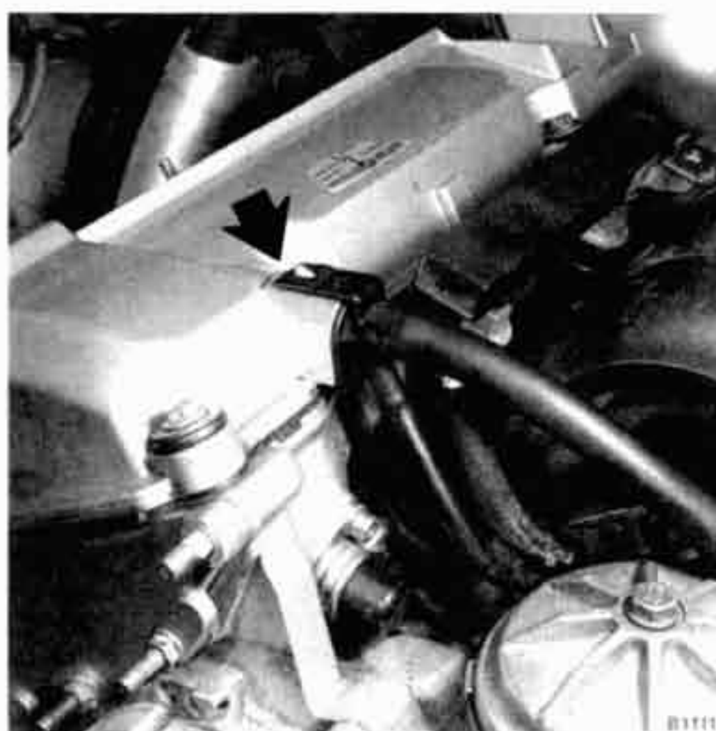
Fig. 3. Crankcase ventilation hose fitting (arrow).
