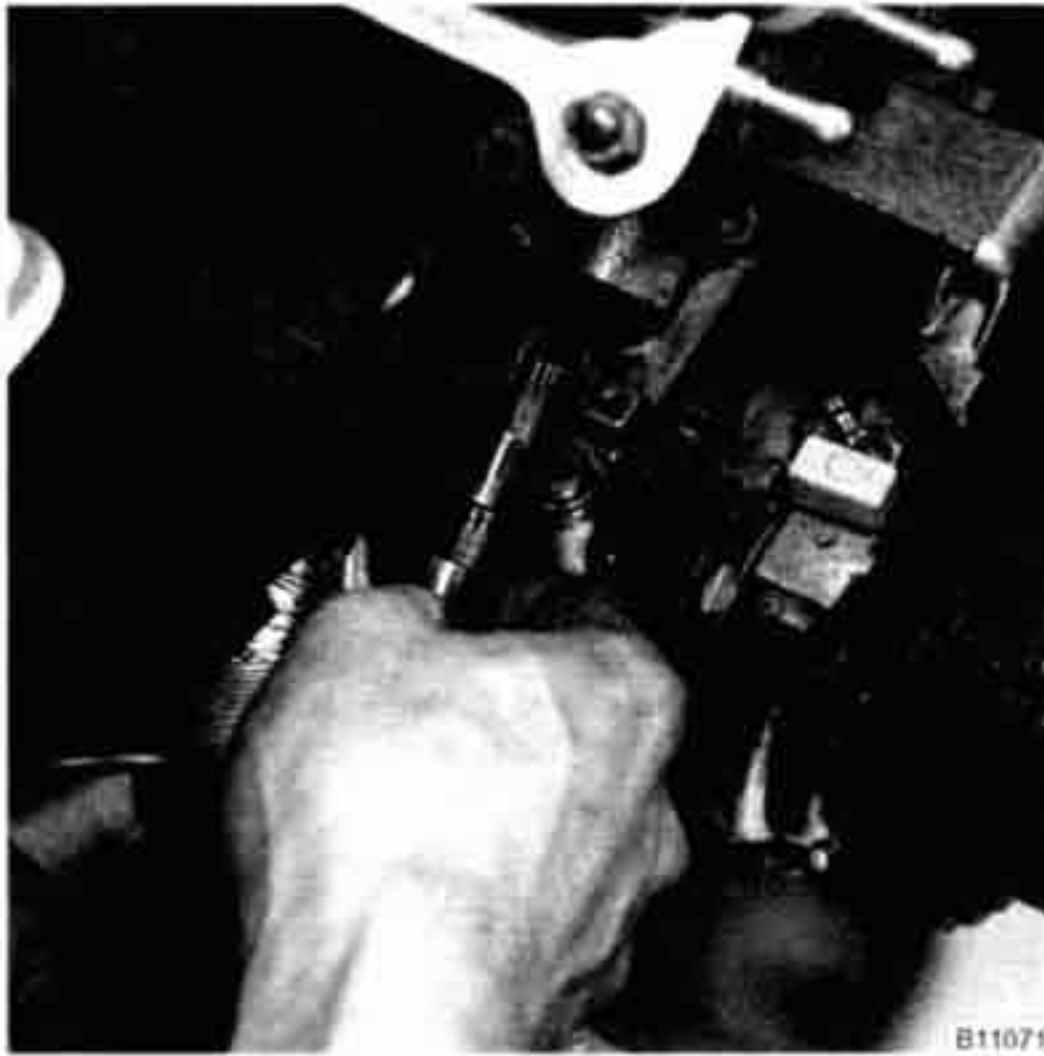
Fig. 31. Primary chain tensioner being installed on 1991 and 1992 cars. Piston cutout must be in position shown to engage chain rail.
