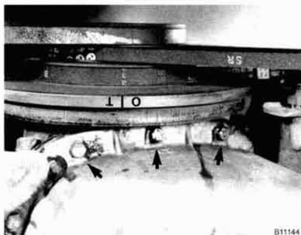
Fig. 26. Front oil pan mounting bolts (arrows) as viewed from below.
