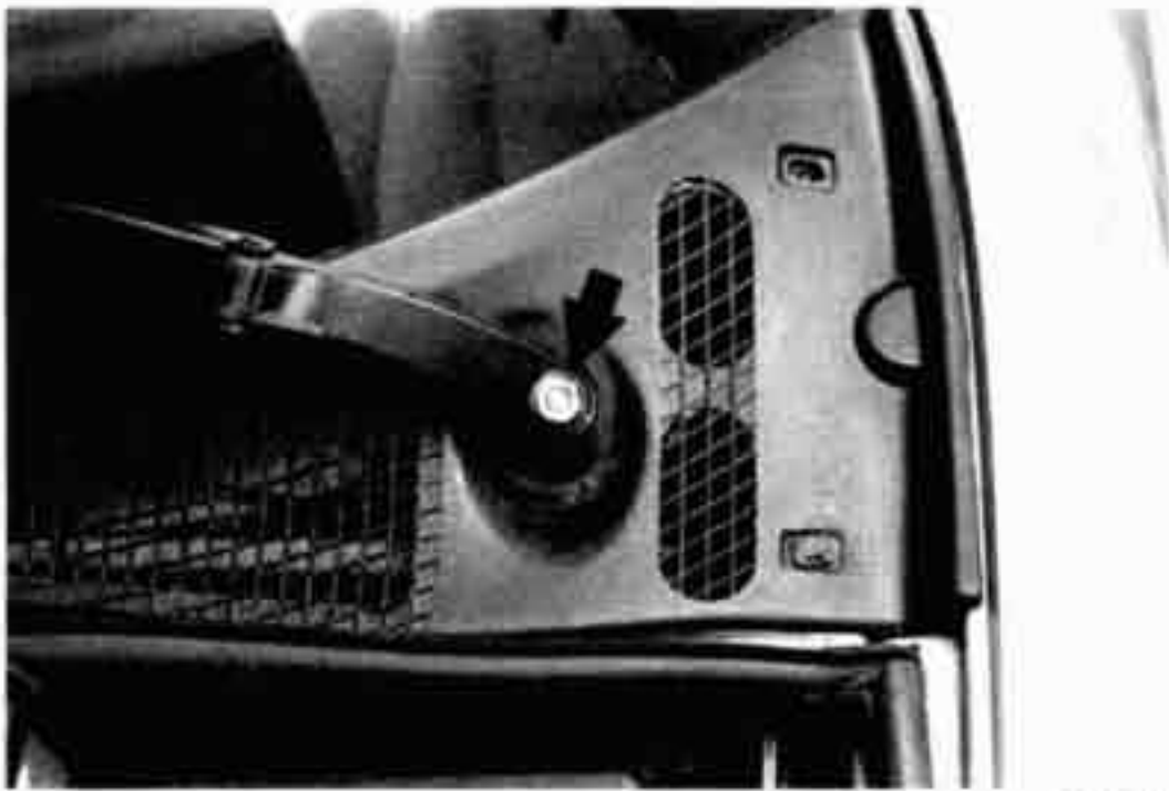
Fig. 5. Wiper arm retaining nut (arrow).
