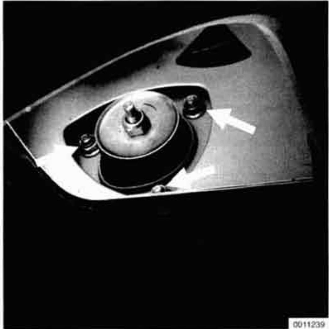
Fig. 4. Rear strut upper mounting nuts (arrows).
