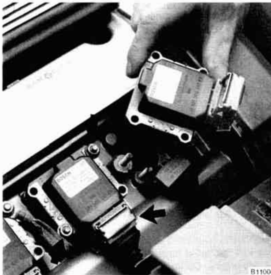
Fig. 6. Remove ignition coils on M50/M60 engines by disconnecting harness connector and removing mounting nuts (arrows).
