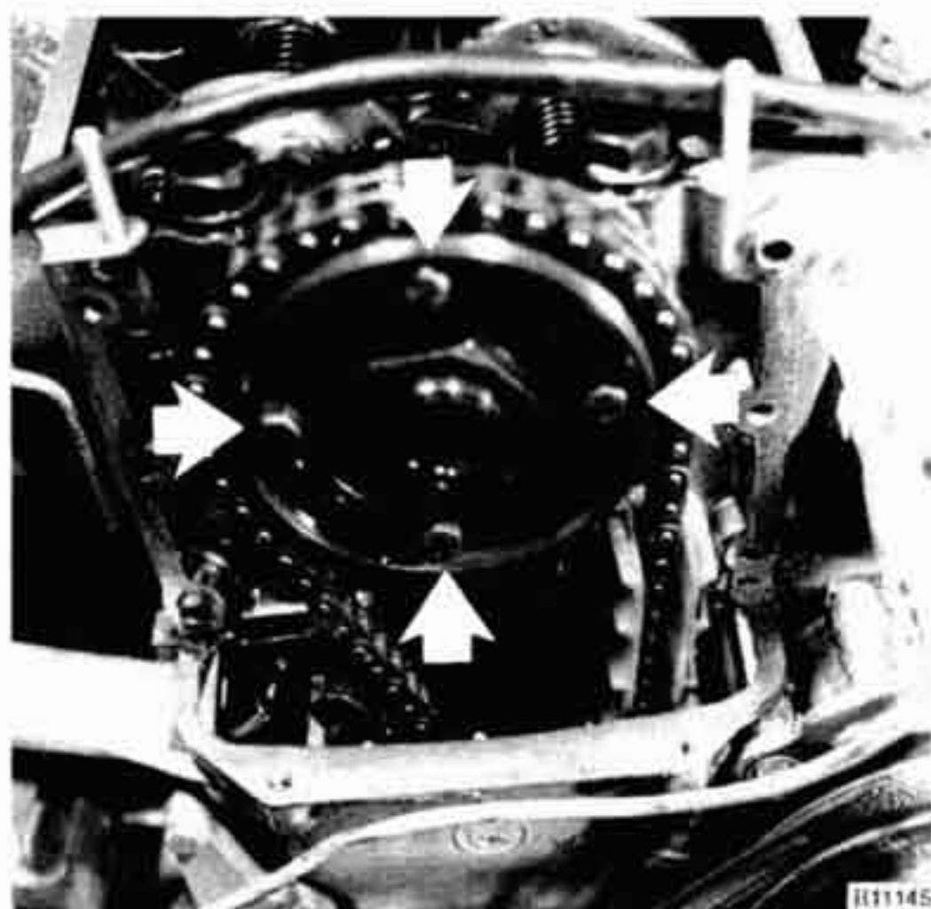
Fig. 27. Camshaft sprocket mounting bolts (arrows).
