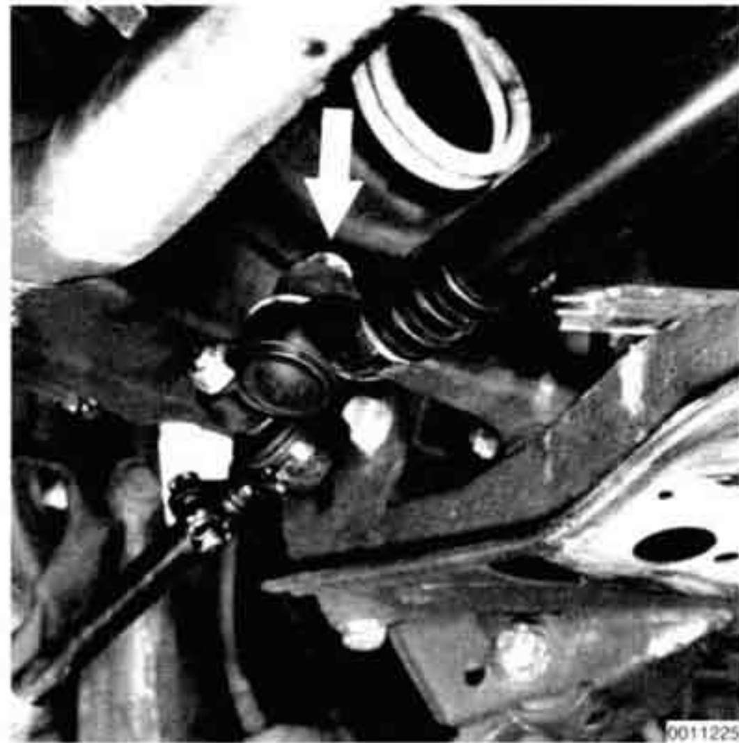
Fig. 4. Center tie rod to pitman arm nut (arrow). Discard self-locking nut.
