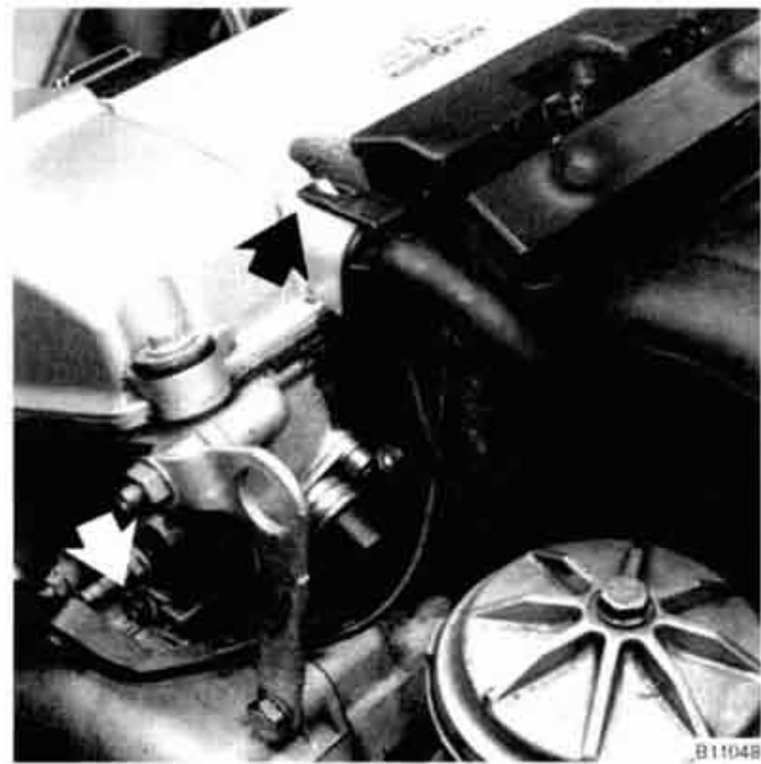
Fig. 9. Crankcase ventilation hose fitting and ground wire (arrows) to be disconnected and removed.
