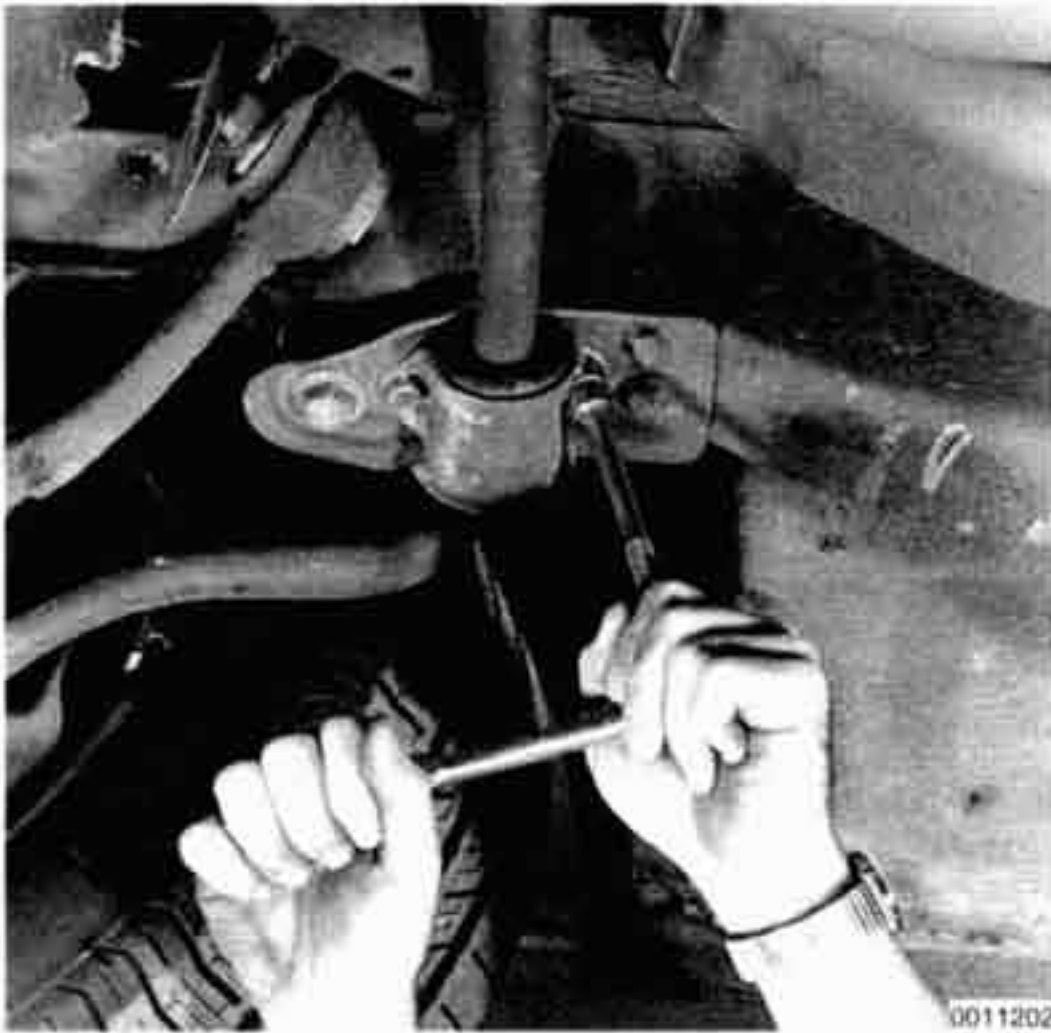
Fig. 13. Stabilizer-to-crossmember mounting bracket being removed.
