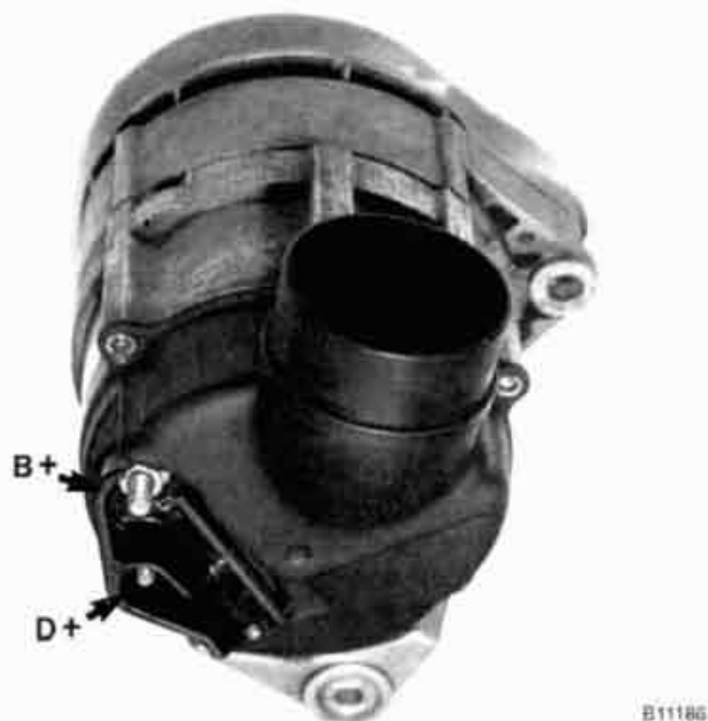
Fig. 3. Alternator terminal designation.
