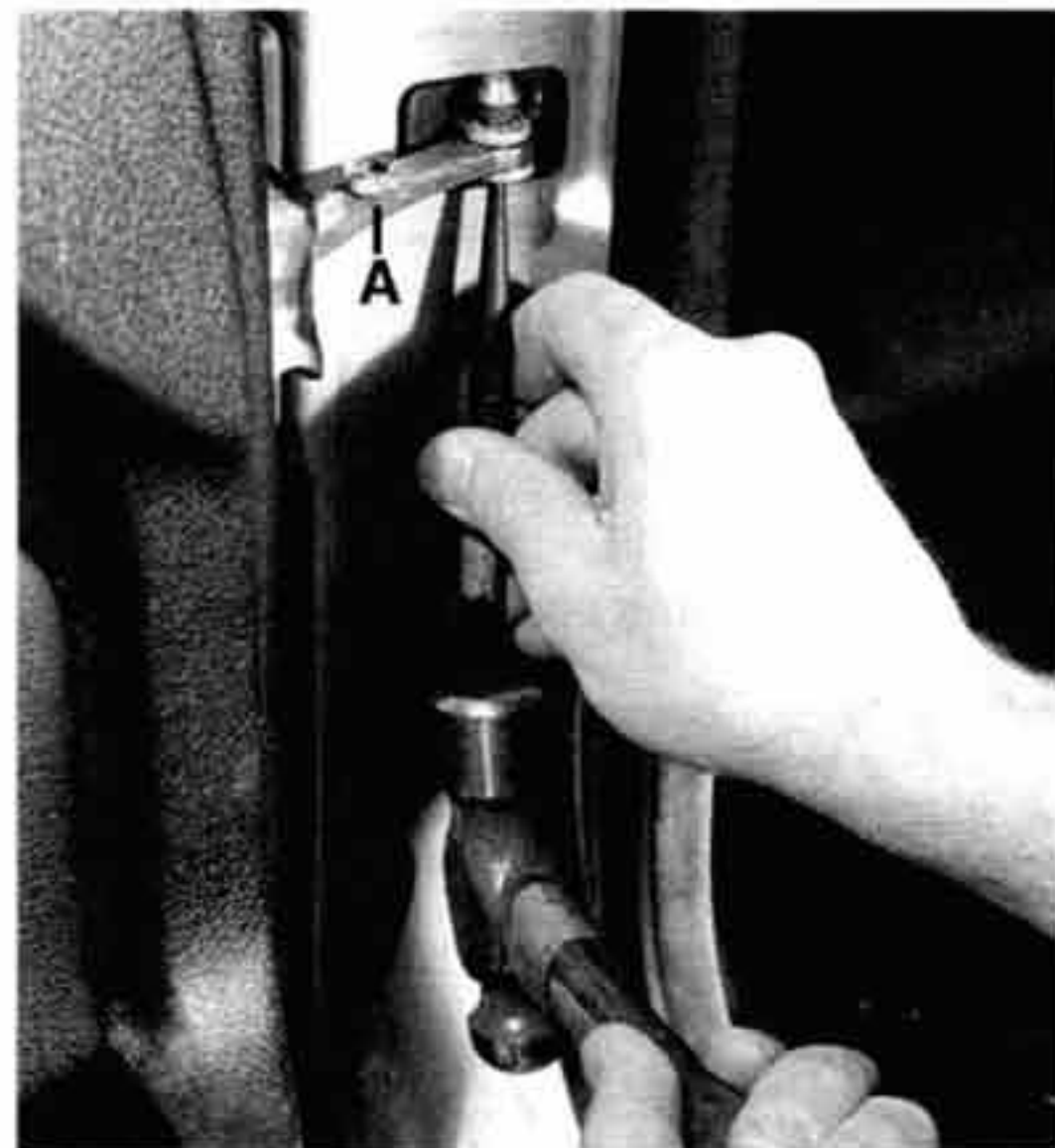
Fig. 2. Door check pin being removed. Pin retaining clip shown at A .
