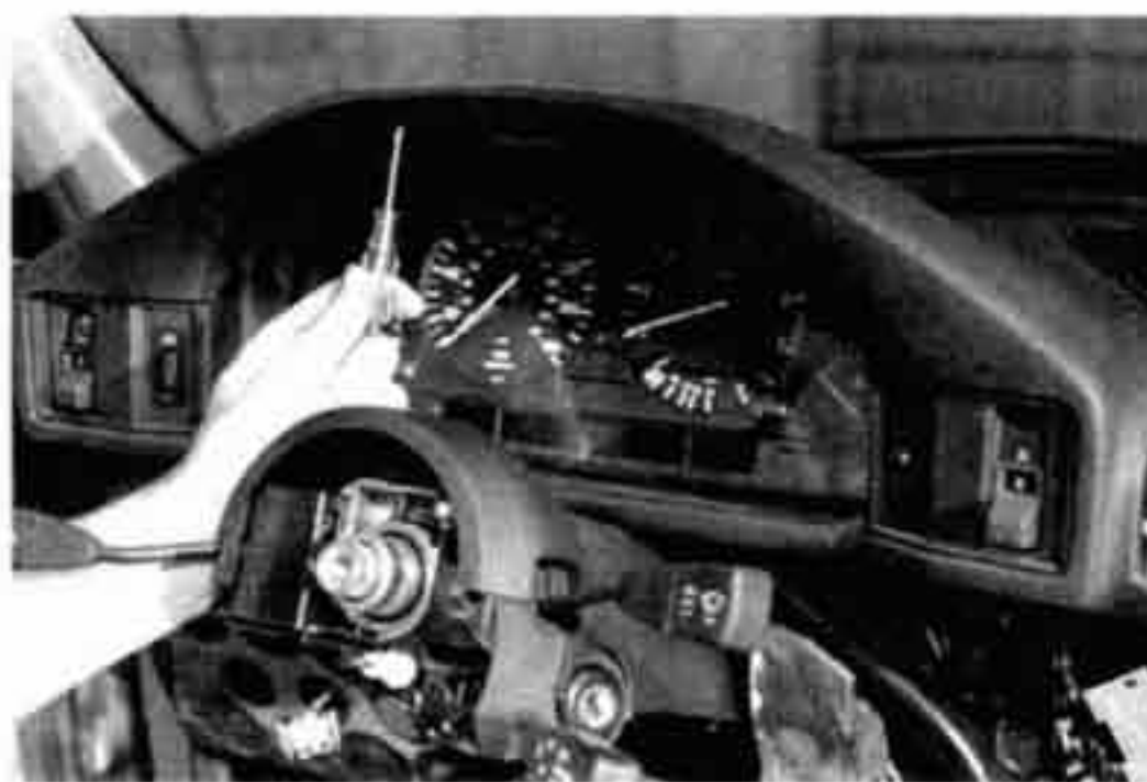
Fig. 1. Instrument cluster retaining screws being removed.
