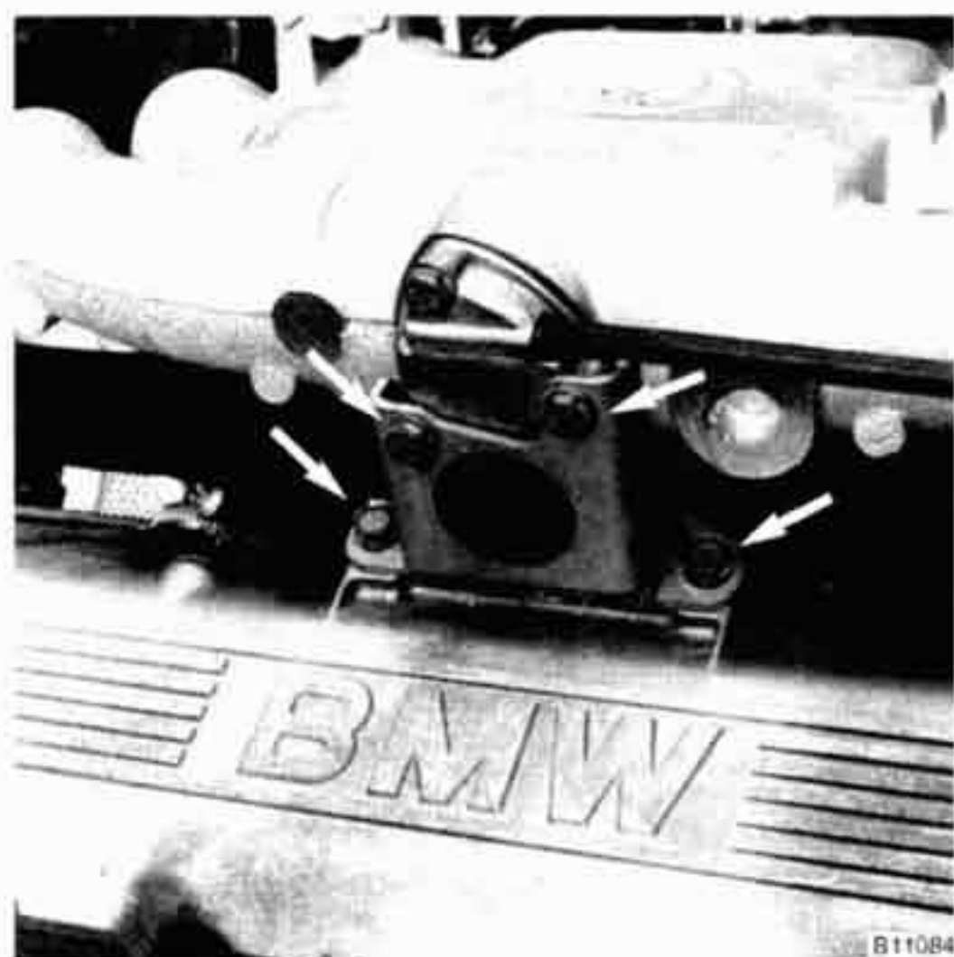
Fig. 1. Intake manifold support bracket mounting bolts (arrows).
