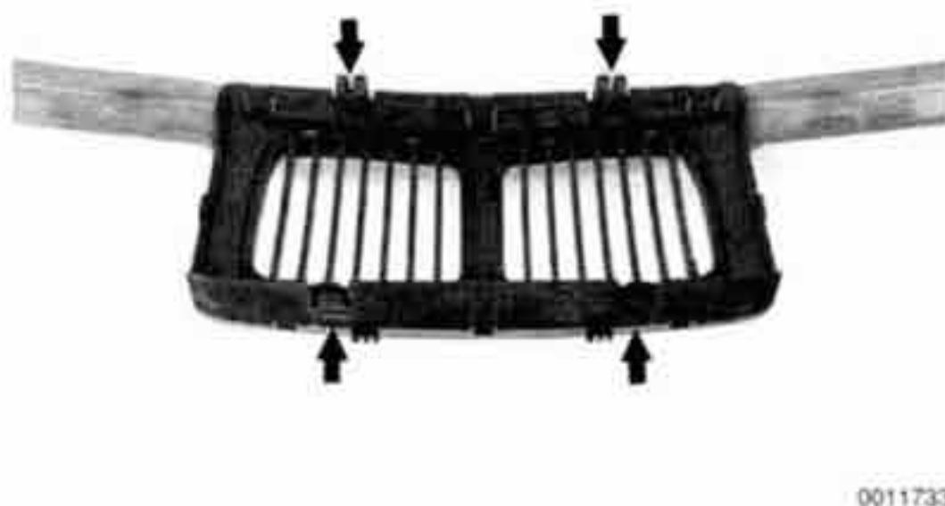
Fig. 8. Center grille retaining clips (arrows)
