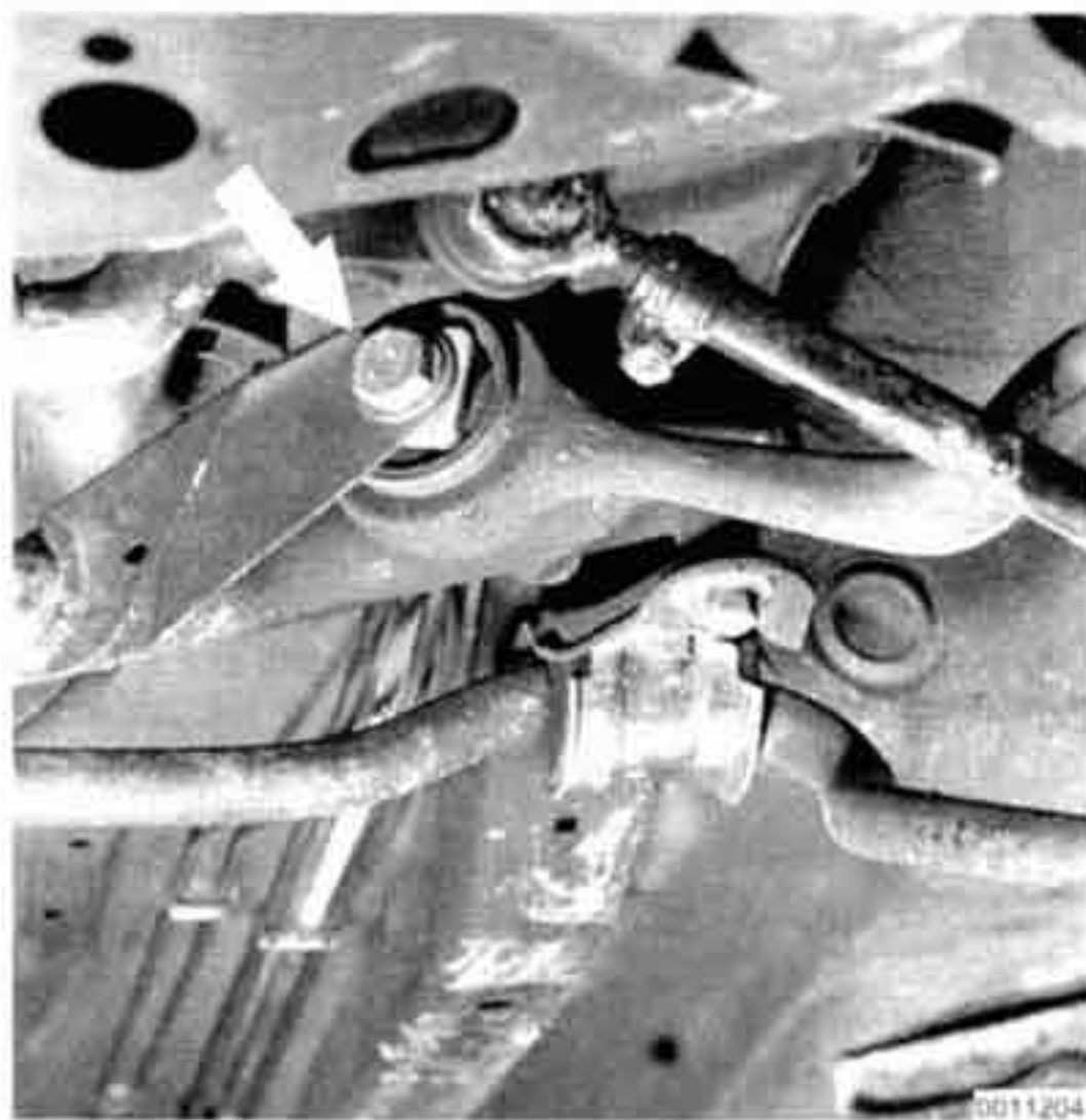
Fig. 15. Thrust arm through-bolt (arrow).
