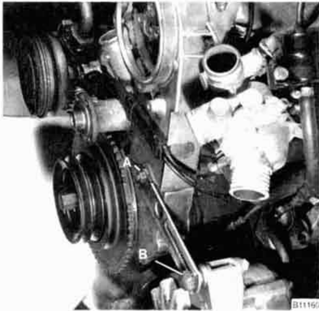
Fig. 2. Remove alternator bracket by removing mounting nut (A) and alternator tensioning bolt (B).
