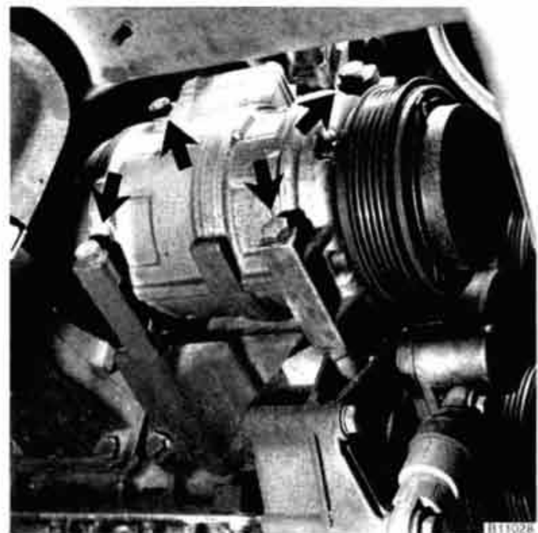
Fig. 20. A/C compressor mounting bolts (arrows).
