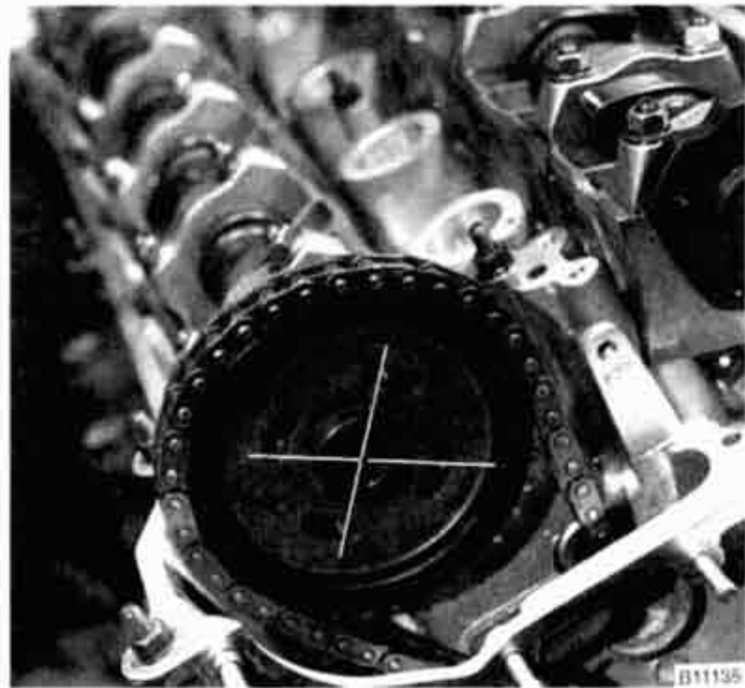
Fig. 19. Primary timing chain sprocket correctly aligned to exhaust camshaft. Elongated sprocket holes should be aligned to left side of threaded camshaft holes.
