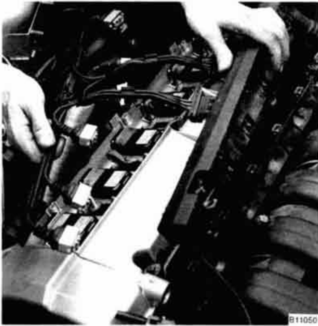
Fig. 21. Injector wiring harness duct being removed from M50 engine.
