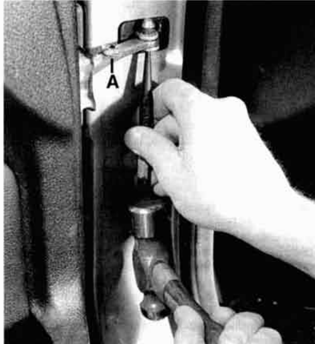
Fig. 17. Door check pin being driven out. Pin locking clip shown at A.
