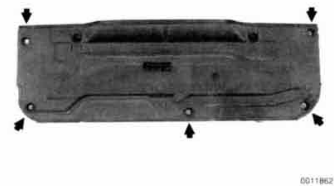
Fig. 1. Bulkhead splash shield retaining screws (arrows).
