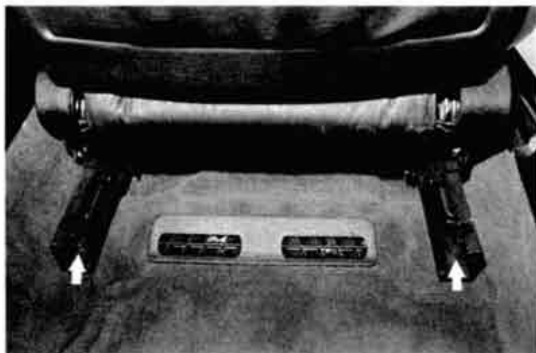
Fig. 1. Front seat mounting bolts (arrows).
