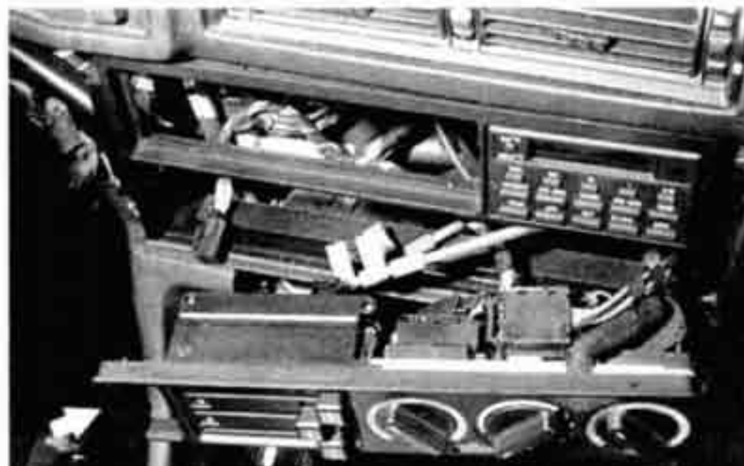
Fig. 5. Remove heater control panel by prying out from left side (arrow).
