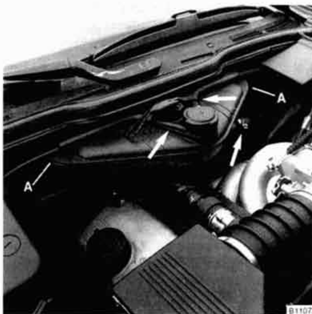
Fig. 32. Coolant reservoir hoses and connectors to be disconnected (arrows). Remove mounting bolts at A to remove reservoir.
