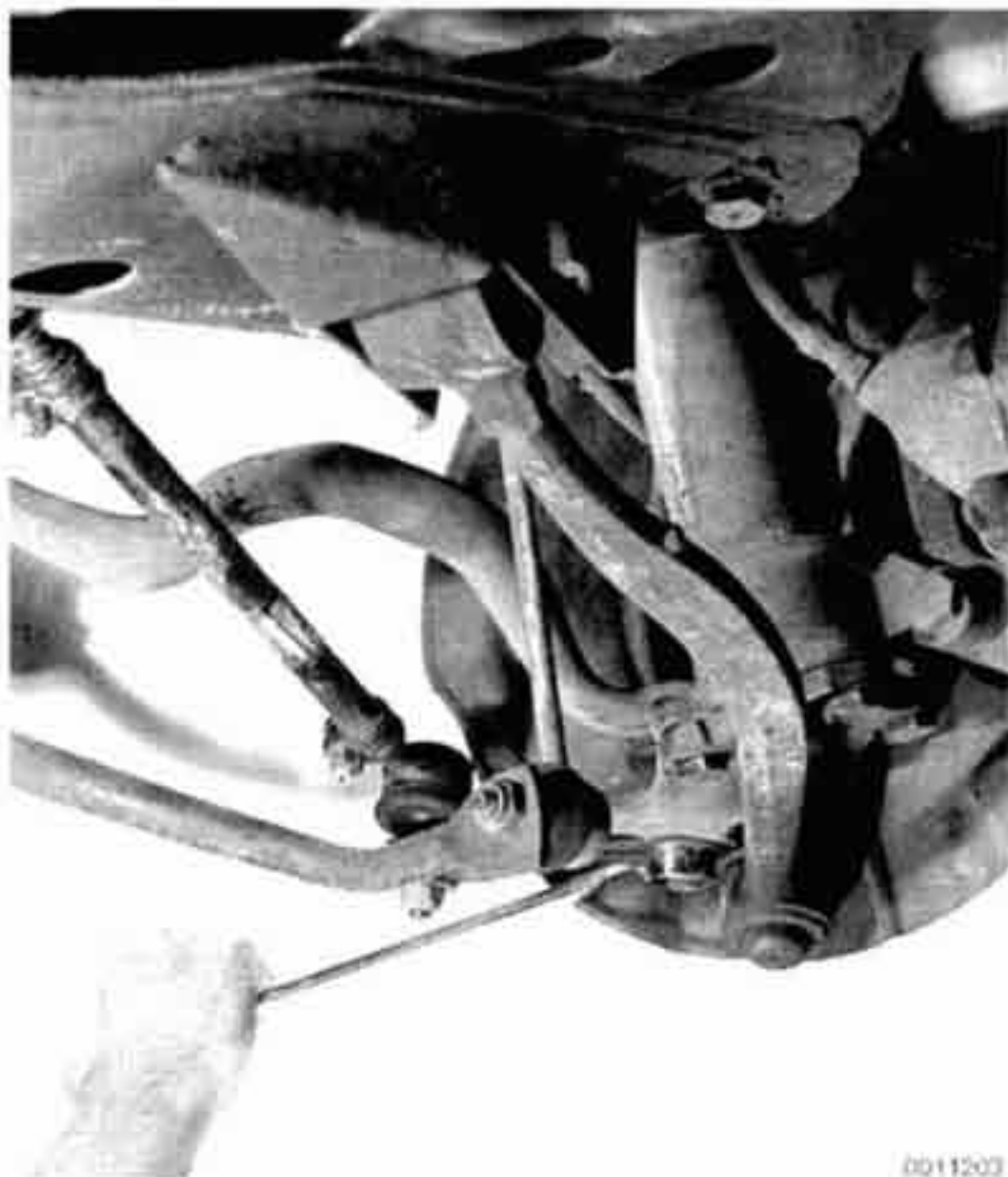
Fig. 14. Thrust arm ball joint being removed from steering arm.
