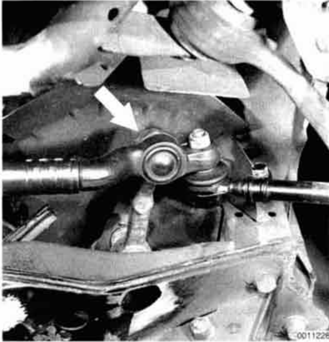
Fig. 8. Idler arm-to-center tie rod self-locking nut (arrow).
