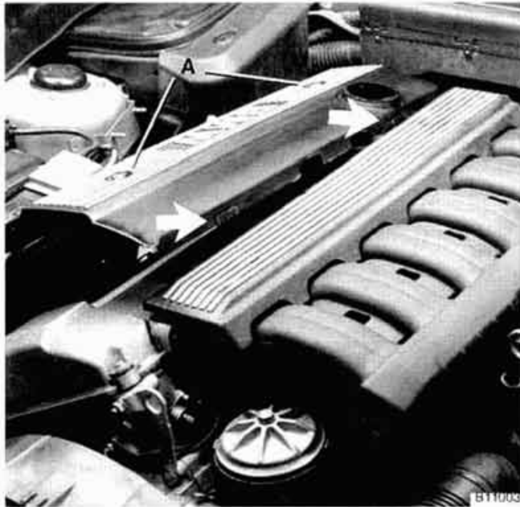
Fig. 5. Remove cover on M50 engine by prying off nut covers and removing nuts (A). Be careful not to let rubber insulators fall off as cover is removed (arrows). M60 engine is similar.
