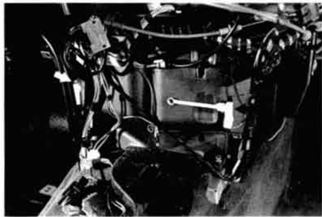
Fig. 13. Left and right heater core temperature sensors (arrows). Right side sensor shown removed.
