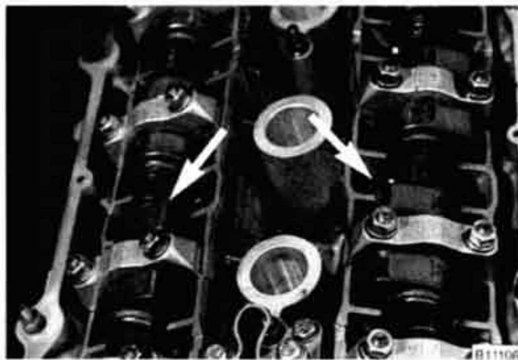
Fig. 28. Camshaft correctly positioned for reassembly so that cylinder no. 1 lobes face each other.
