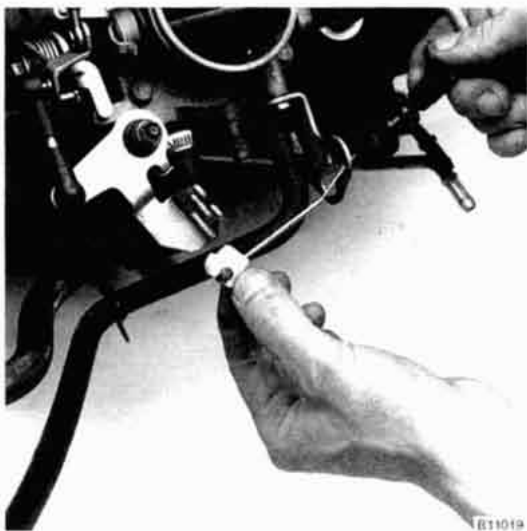
Fig. 13. Throttle cable being removed. Disconnect cable at lever and pull cable with grommet from bracket.
