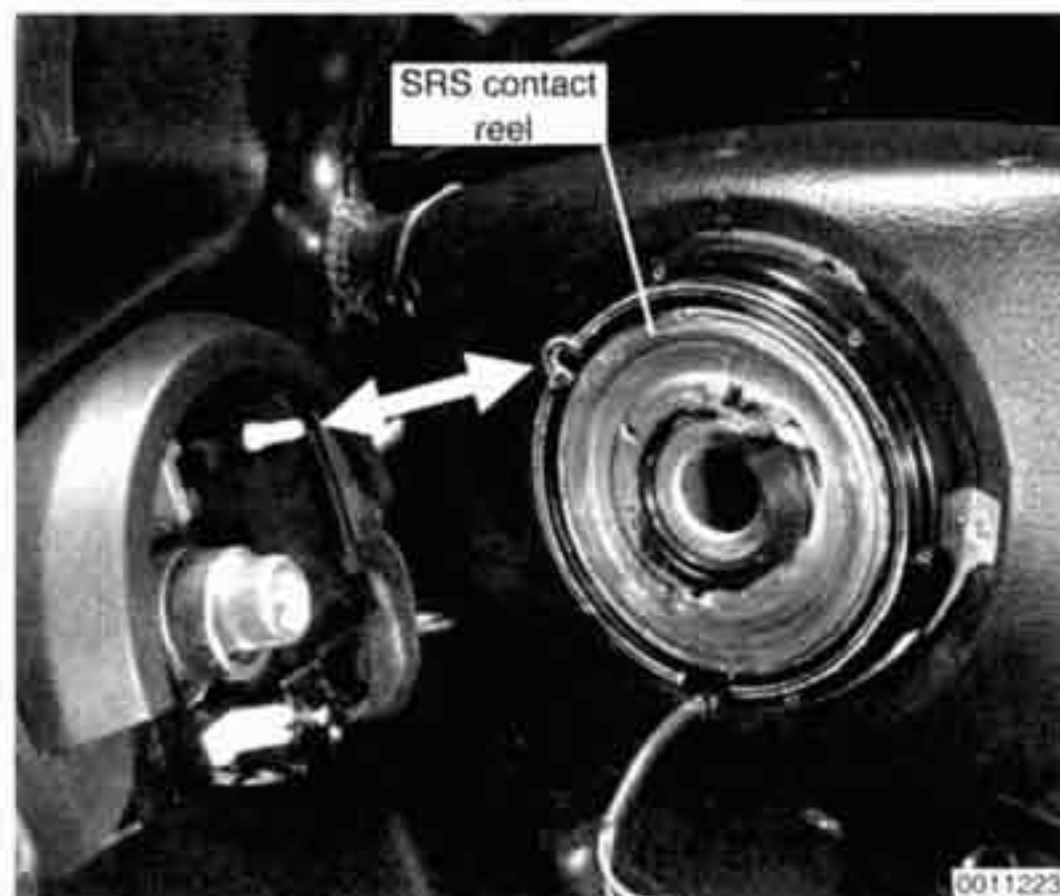
Fig. 1. Install steering wheel so that locking pin in column aligns with cutout in contact reel (arrow).
