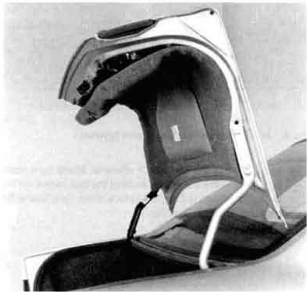
Fig. 6. Trunk lid panel partially removed to access locking drive.
