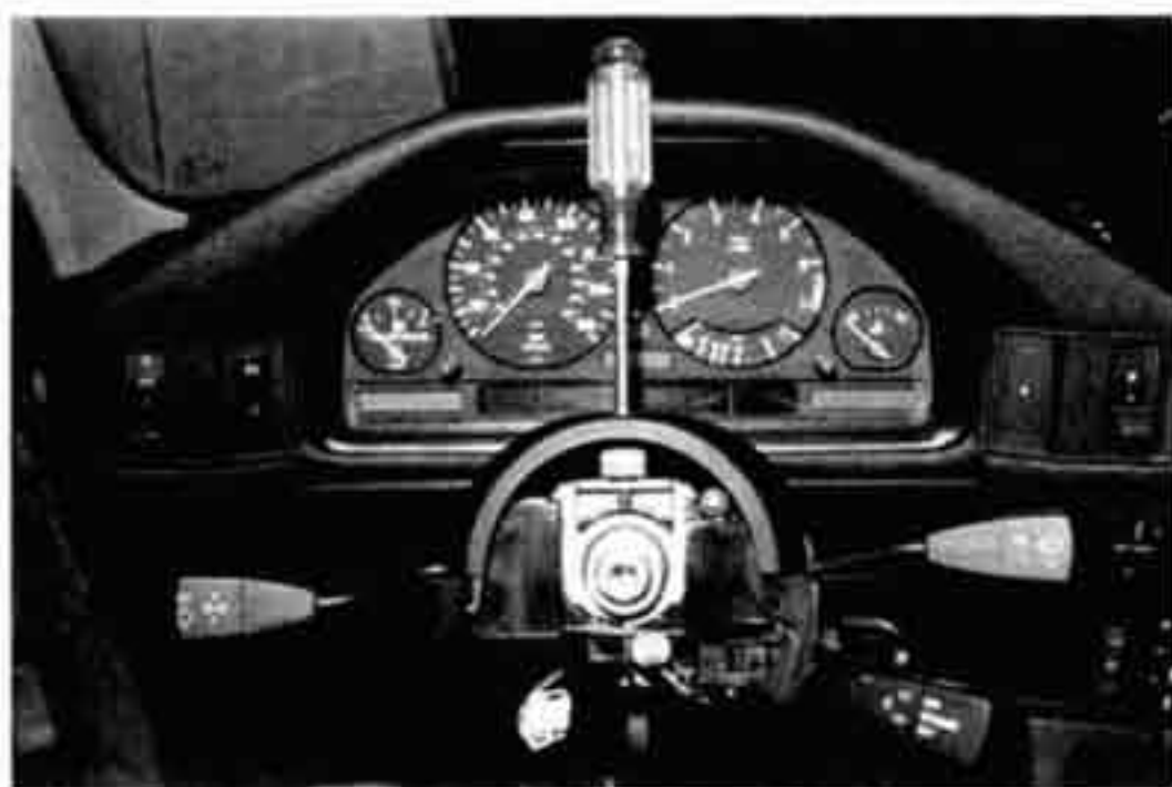
Fig. 1. Upper steering column trim cover retaining screw being removed. Some models may have retaining pins instead of screw.
