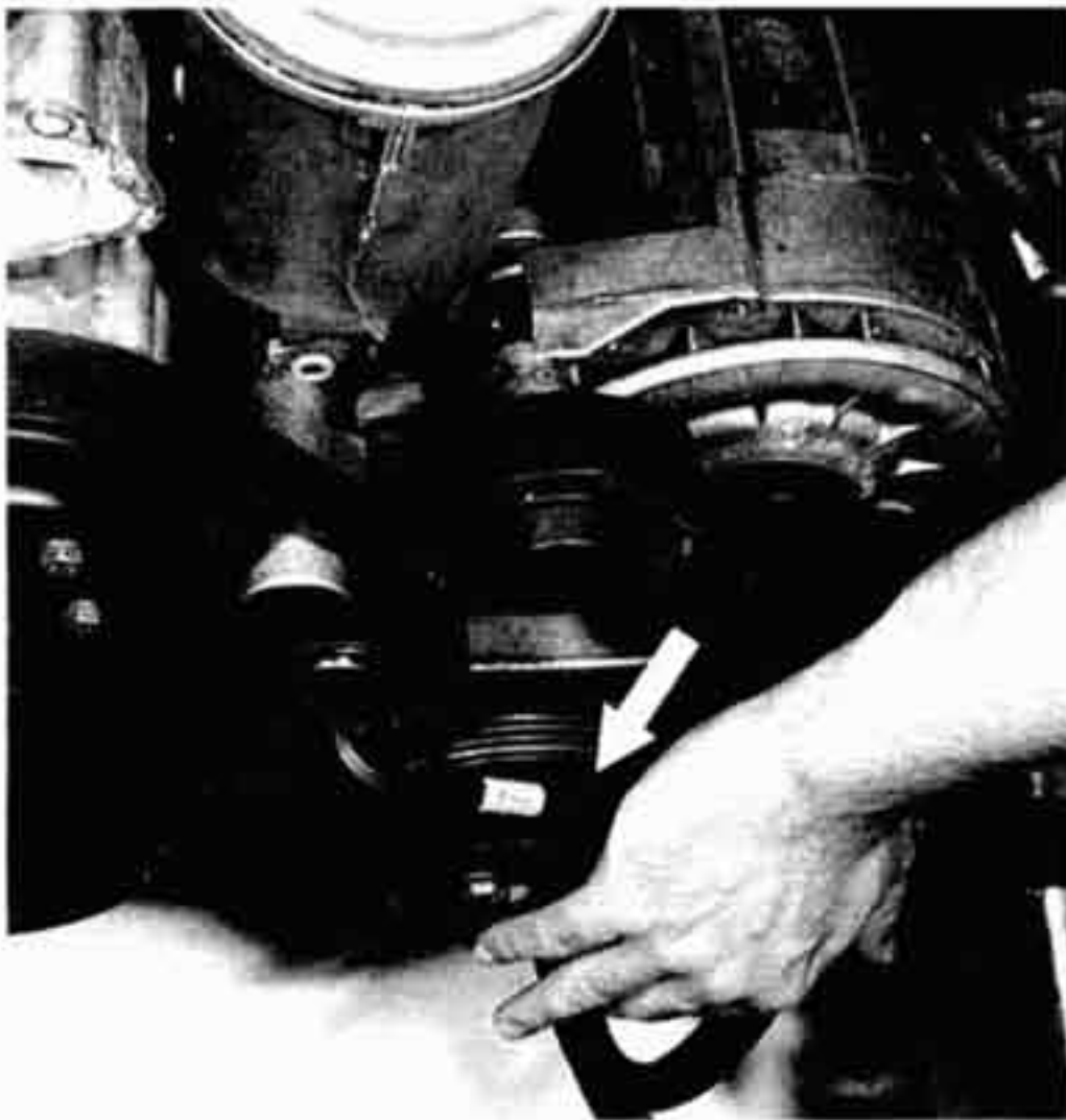
Fig. 5. To remove poly-ribbed drive belt, pry cover from front of tensioner. Then using 8mm hex key, turn tensioner clockwise (arrow) to release tension and slip belt off pulleys.
