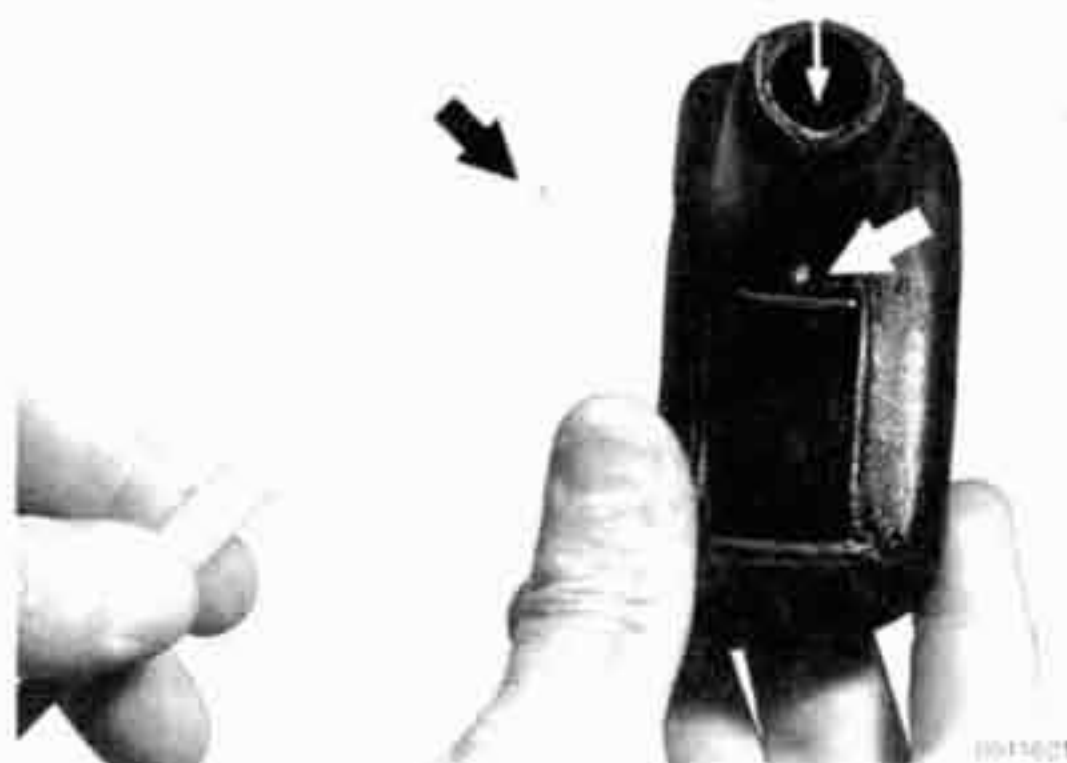
Fig. 11. Engage release button pin to hole in pull rod.
