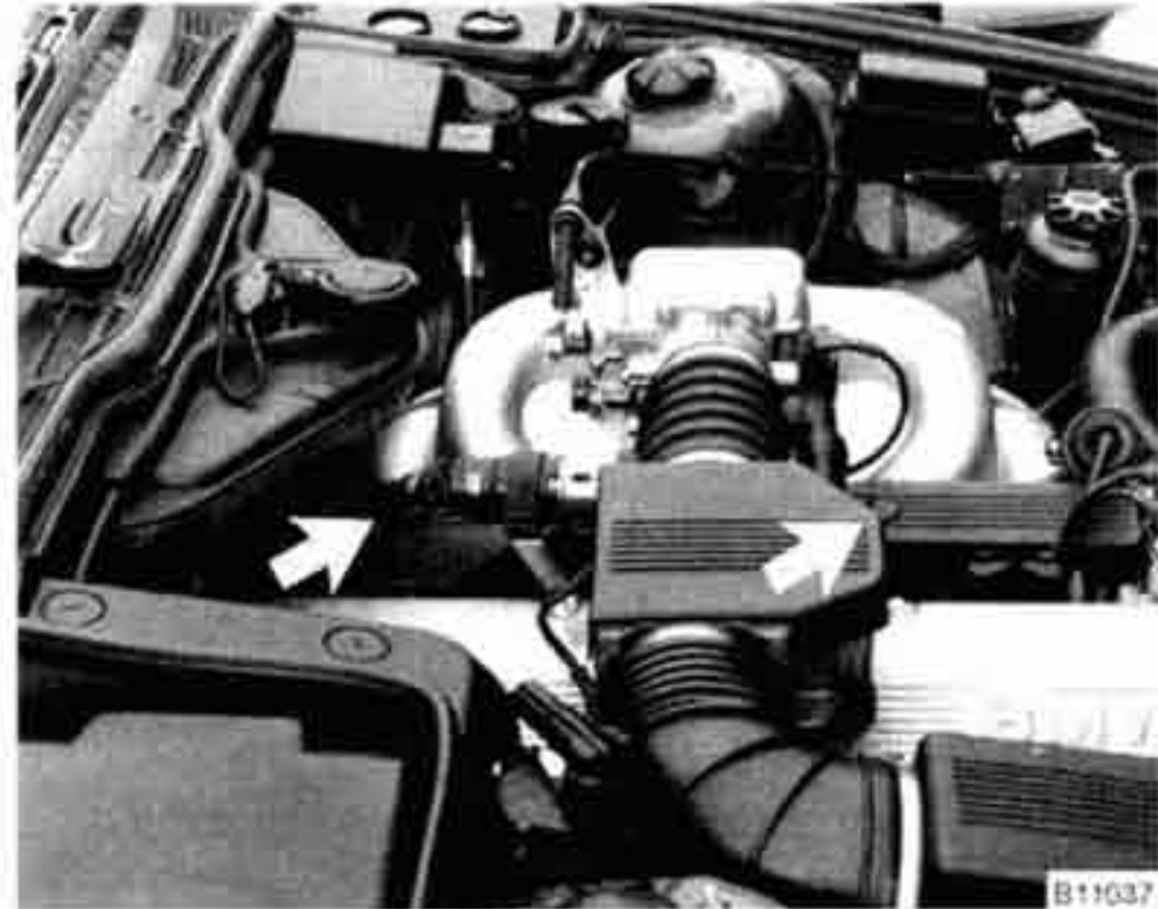
Fig. 29. Wiring harness bracket cover plugs (arrows).
