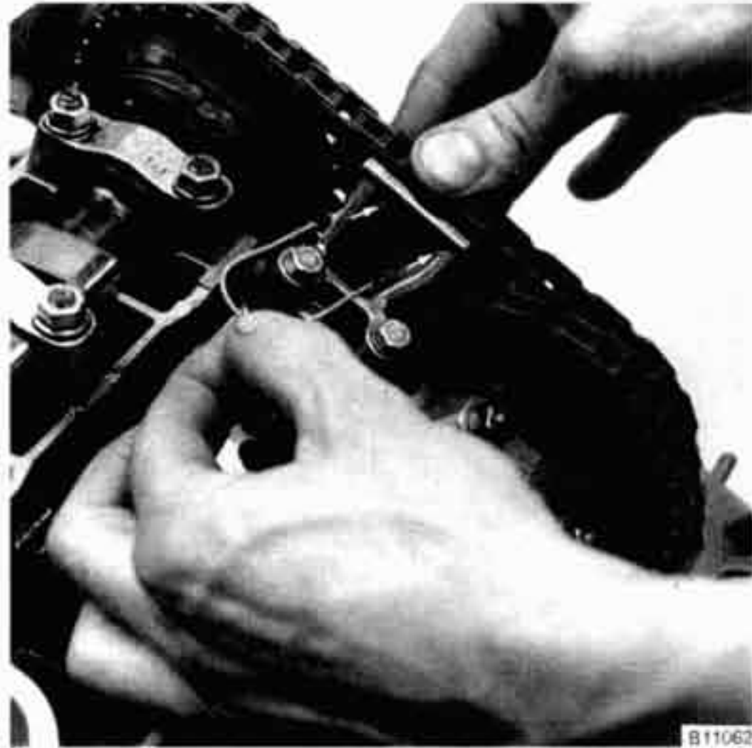
Fig. 22. Secondary timing chain tensioner being locked down. Press tensioner down fully and insert wire through holes (arrow).
