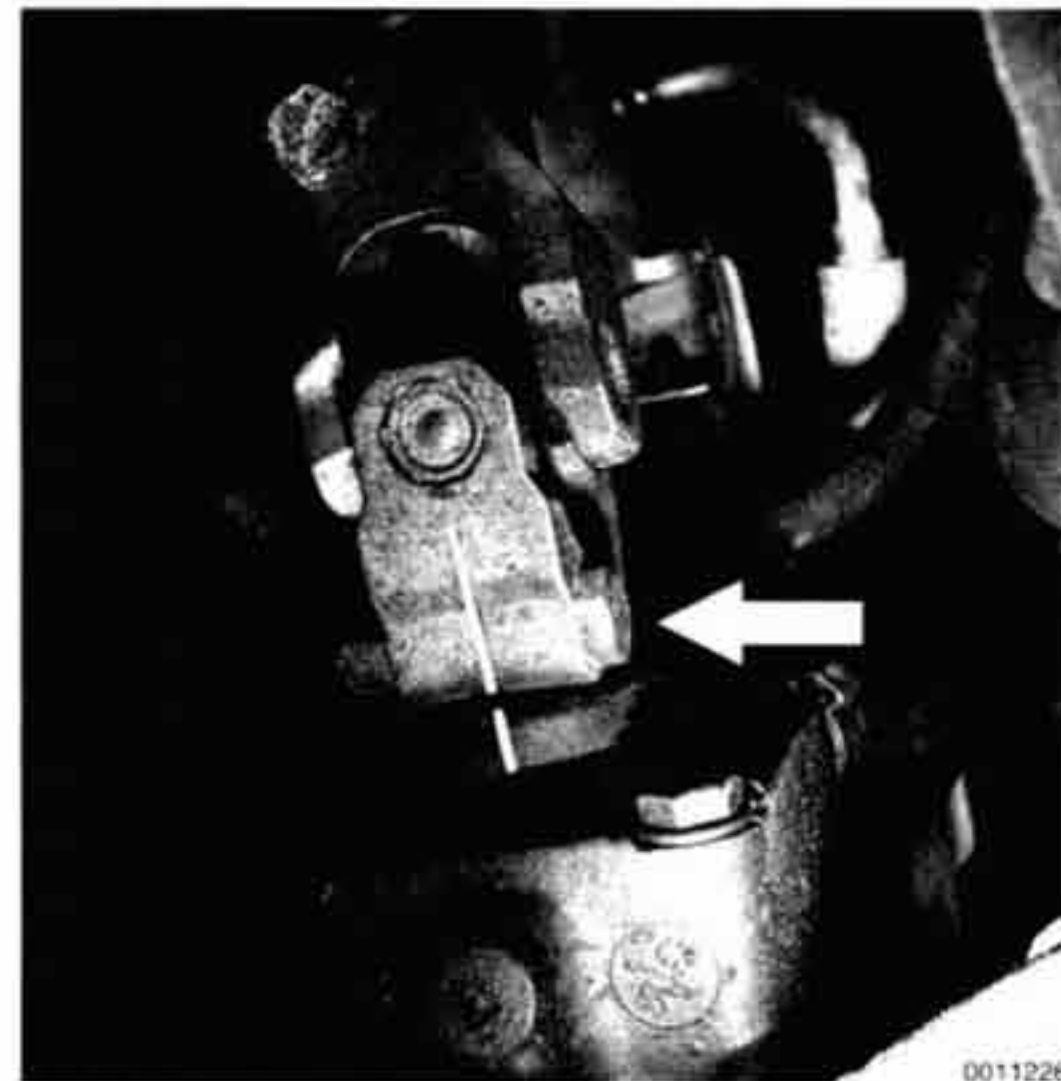
Fig. 5. Universal joint lower clamping bolt (arrow).
