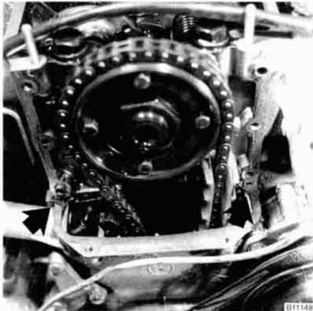
Fig. 31. Apply sealer (arrows) to corners before installing chain cover.
