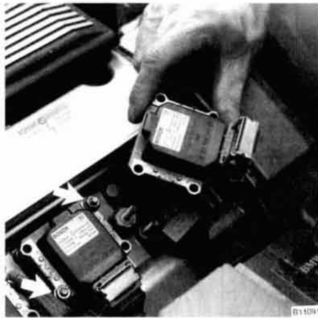
Fig. 12. Ignition coil being removed.
