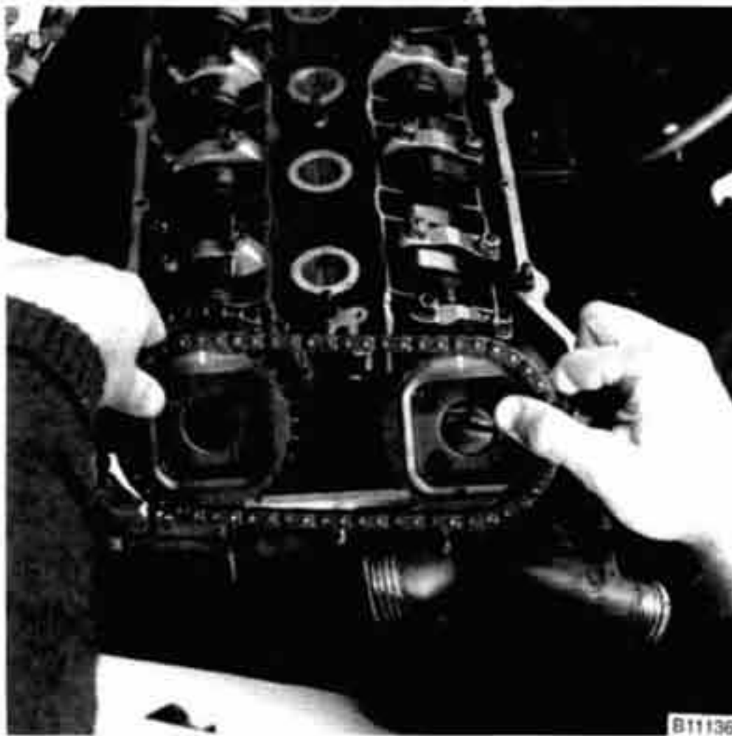
Fig. 20. Secondary chain sprockets and chain being installed on non-VANOS engine. Attach sprockets with arrows pointing up and elongated holes centered.
