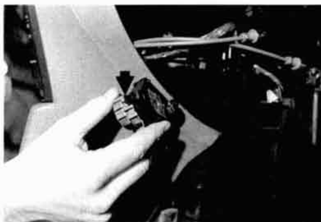
Fig. 16. Air distribution flap stepper motor mounting clip (arrow). Release clip and tilt motor out of housing.
