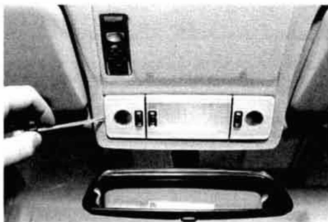
Fig. 9. Dome light assembly being removed.
