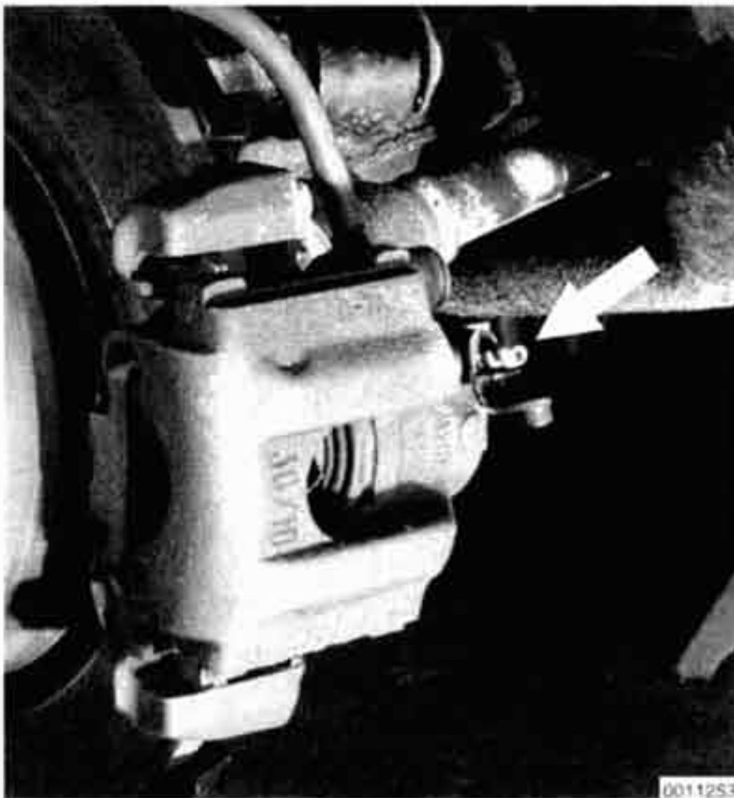
Fig. 1. Brake caliper bleeder screw (arrow).
