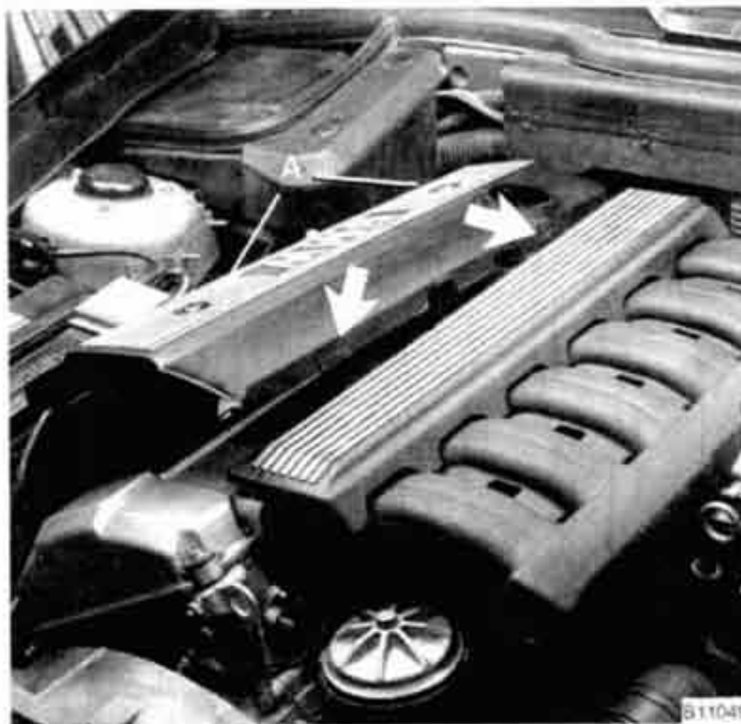
Fig. 27. Remove top engine covers by prying out caps and removing nuts (A). Note rubber gaskets at cover edge (arrows).
