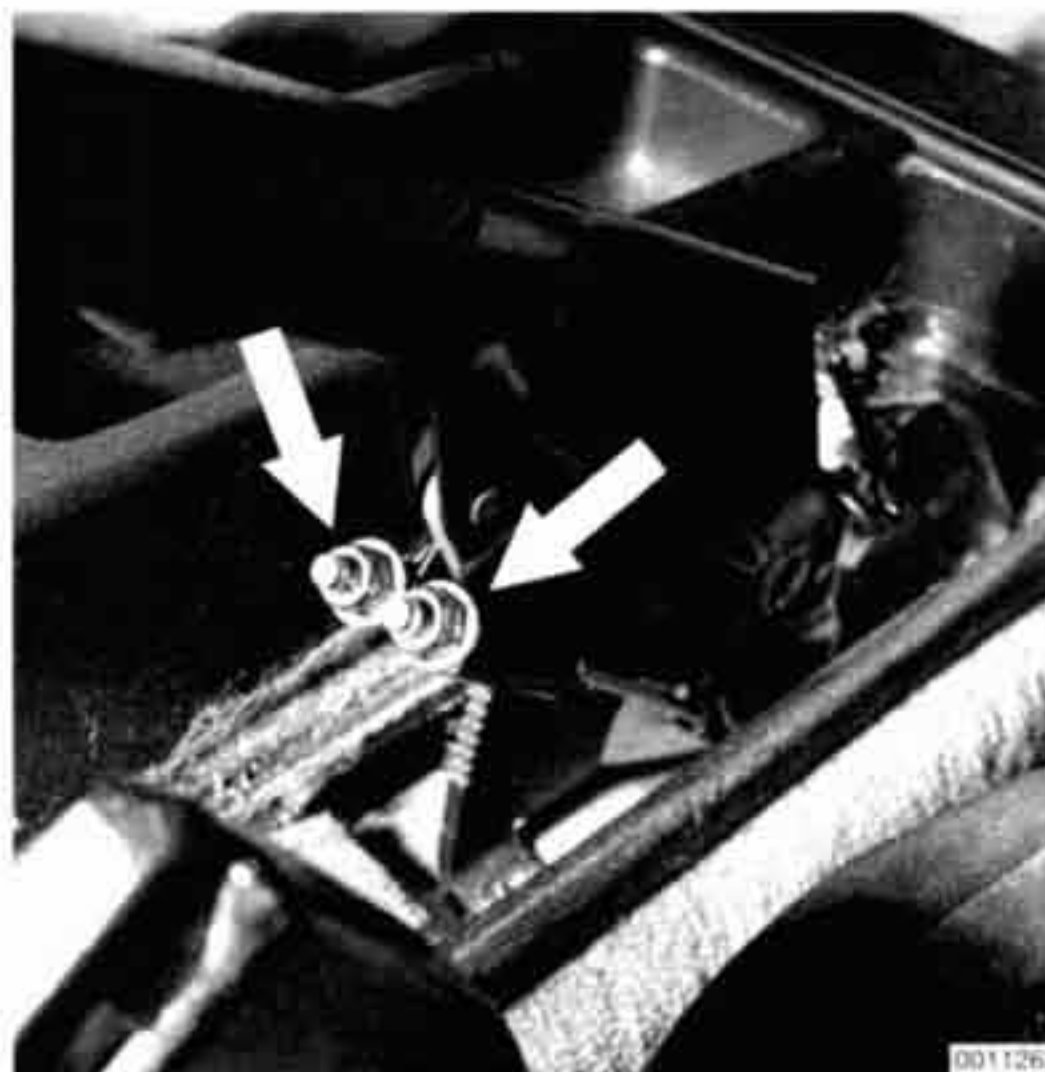
Fig. 16. Parking brake cable adjusting nuts (arrows).
