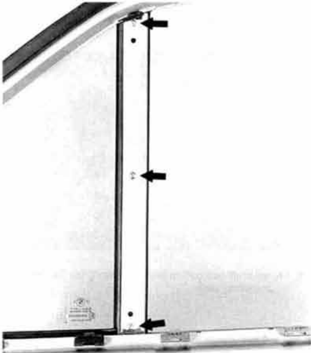
Fig. 6. Rear window guide mounting screws (arrows).
