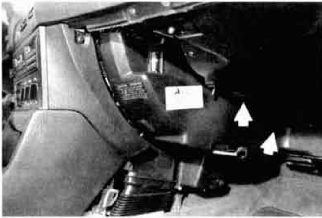
Fig. 5. Slide console trim cover forward and out after removing retaining clip and screw (arrows)
