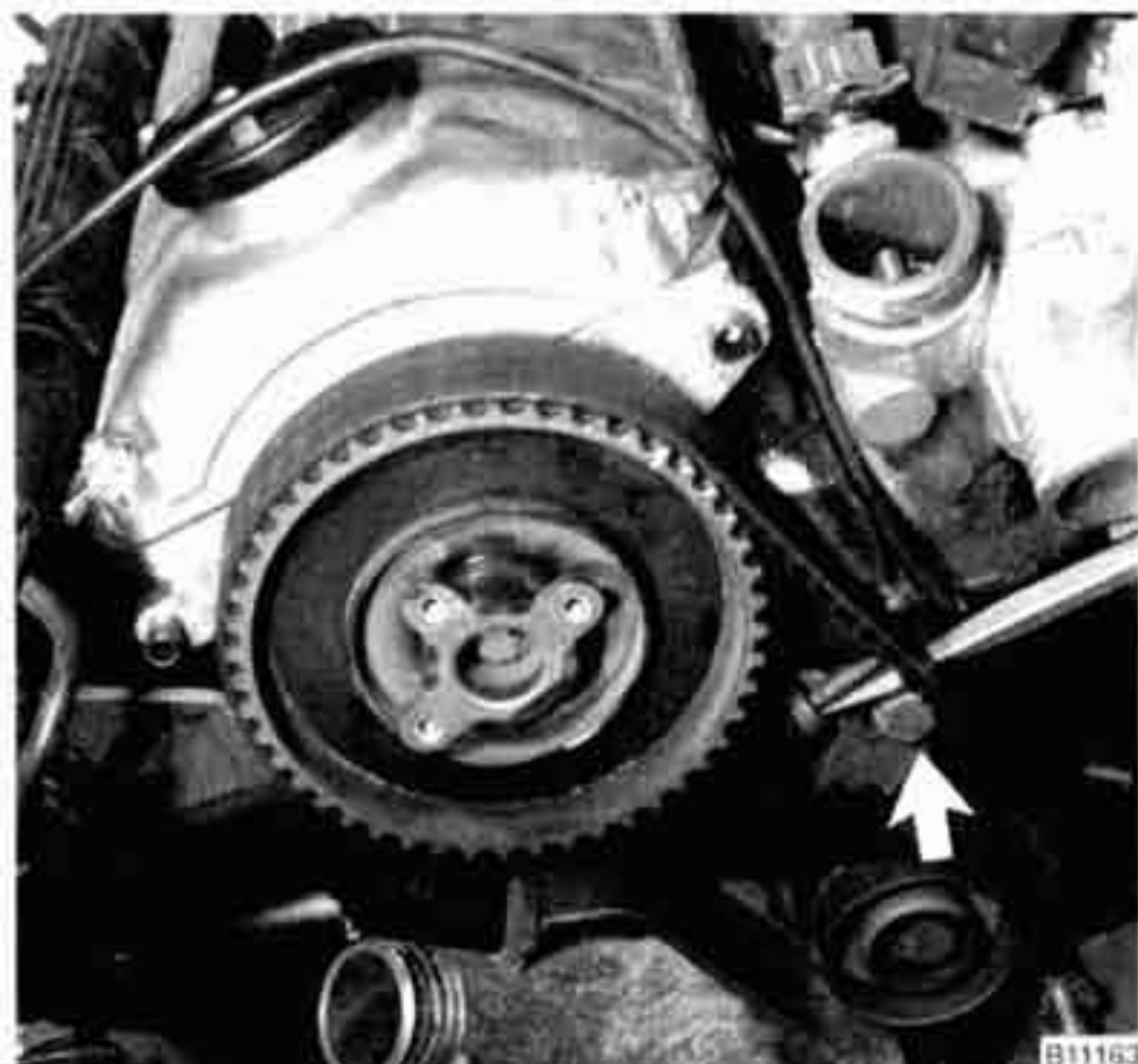
Fig. 5. Push in on the tensioner with screwdriver, then tighten top bolt (arrow).
