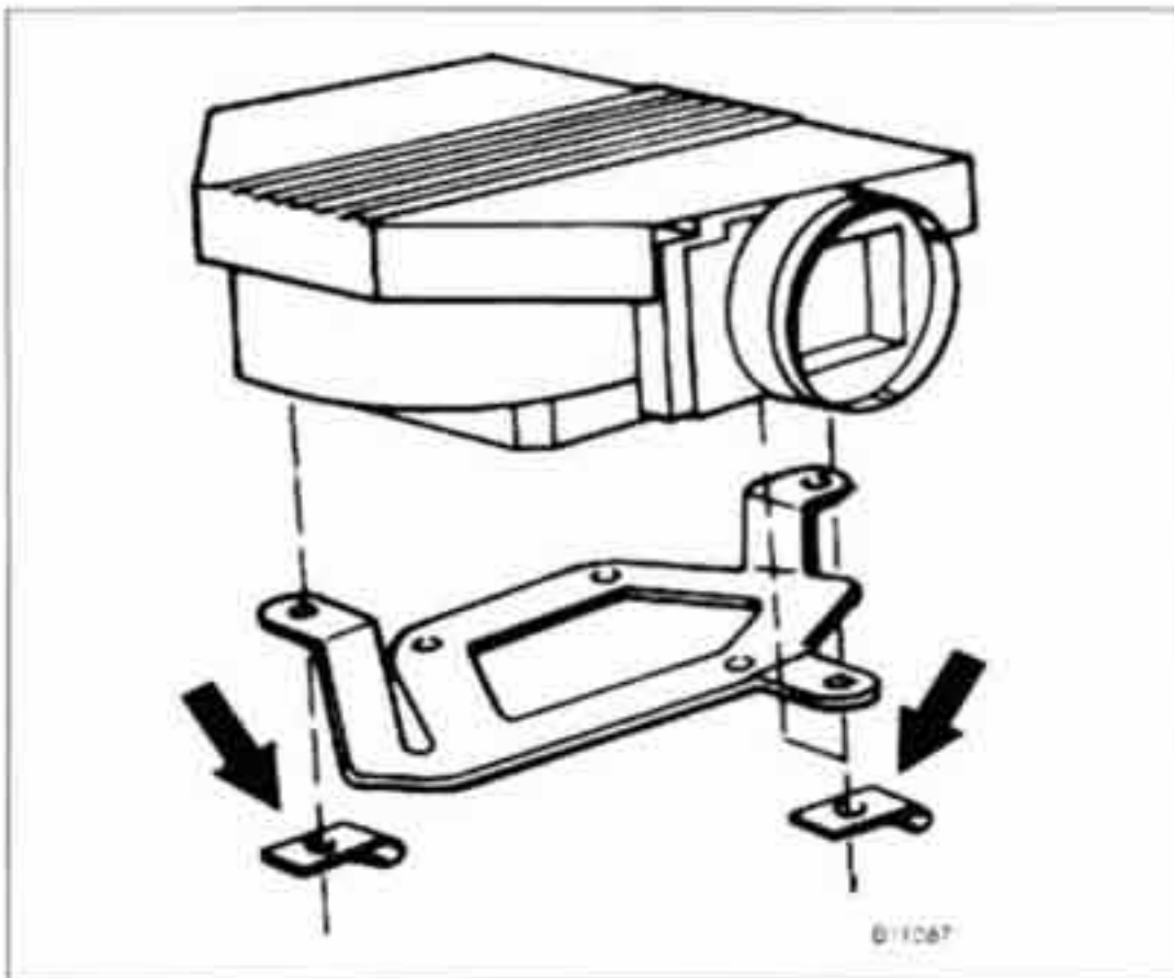
Fig. 5. Air flow sensor mounting clips on M30 engine (arrows).
