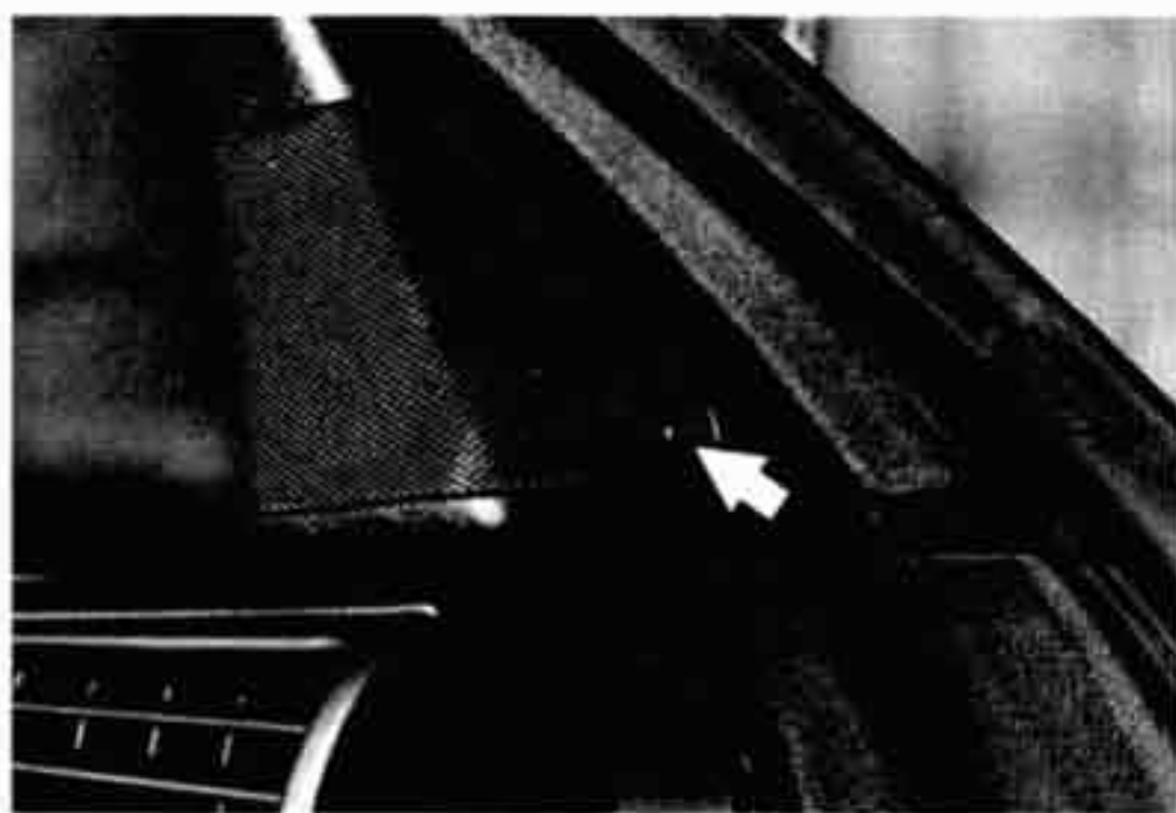
Fig. 5. Door loudspeaker mounting screw (arrow). Pry off plastic cover to access screw.
