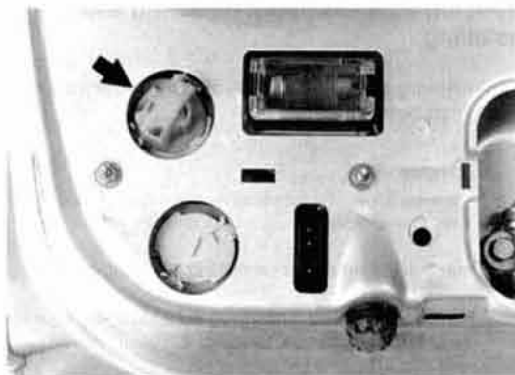
Fig. 10. To remove tail light bulb socket ( arrow ), twist 90° and pull out of lens assembly.
