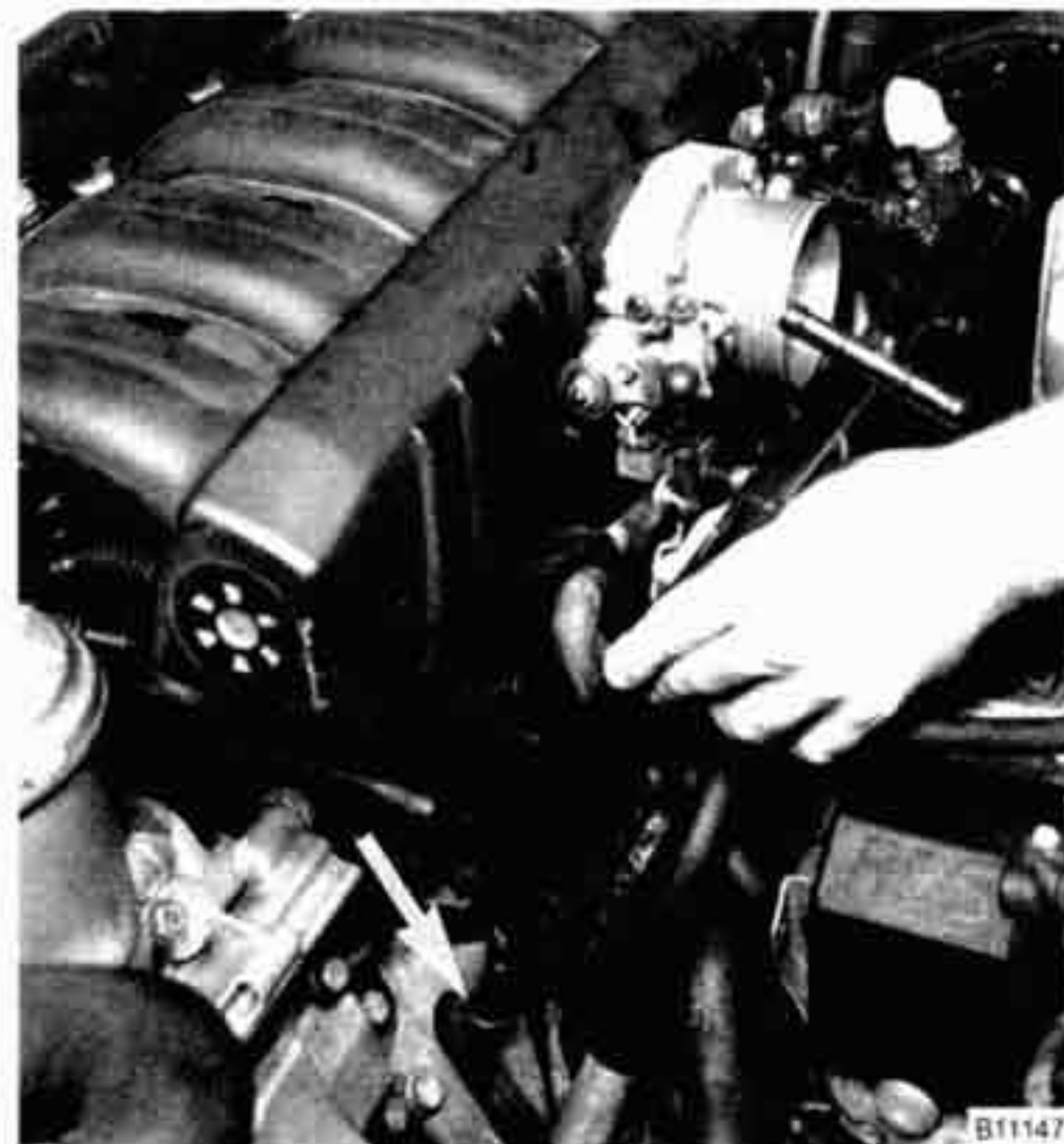
Fig. 7. Oil dipstick guide tube being removed. Use a new O-ring (arrow) during installation.
