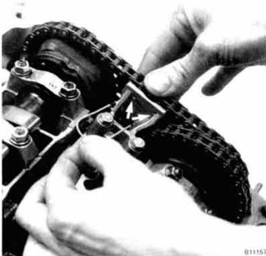
Fig. 39. Secondary timing chain tensioner being locked down. Press tensioner down and insert locking wire through holes (arrow).
