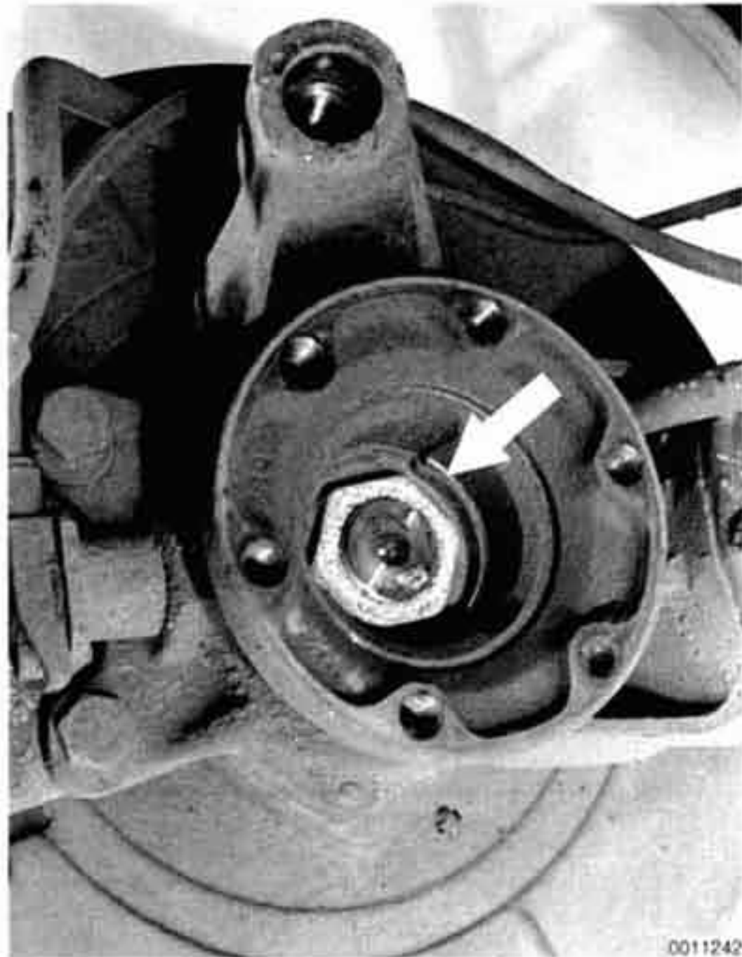
Fig. 7. Drive flange collar nut and lockplate (arrow).
