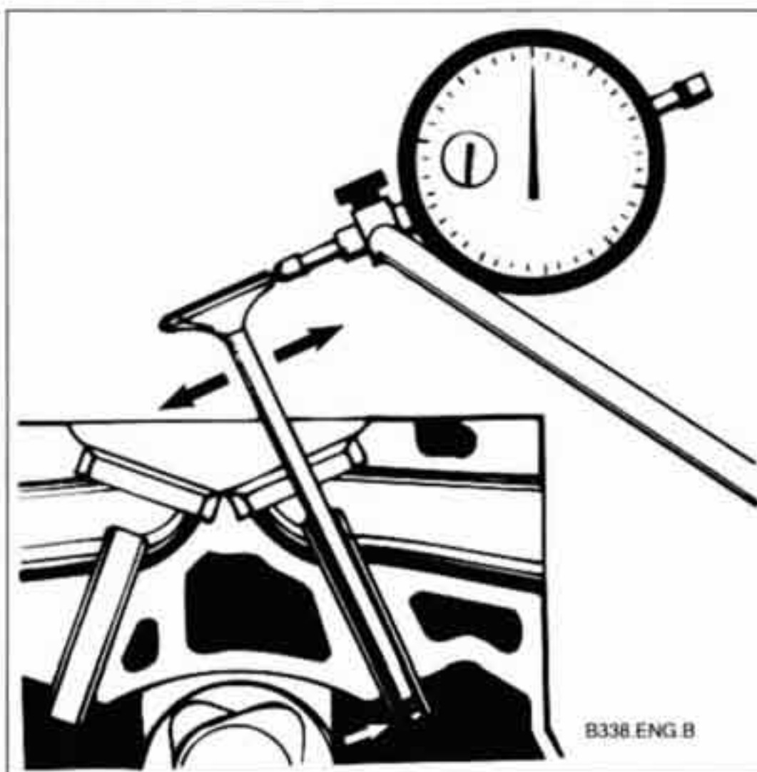
Fig. 39. Valve guide wear being checked with dial indicator. Insert new valve until stem end is flush with end of guide ( white arrow ). See Table f for wear limits.
