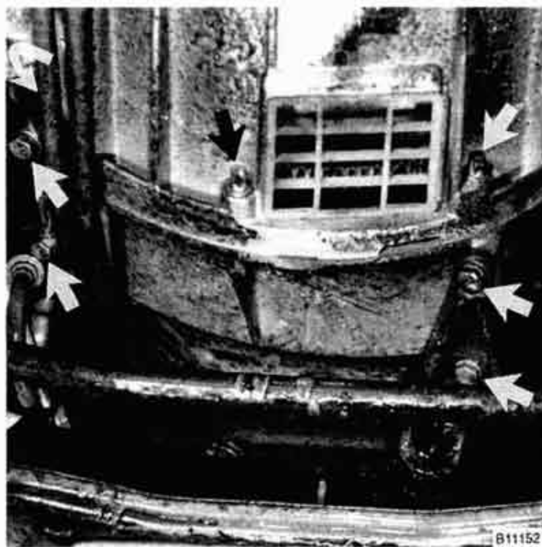
Fig. 4. Bellhousing reinforcement plate mounting bolts (arrows).
