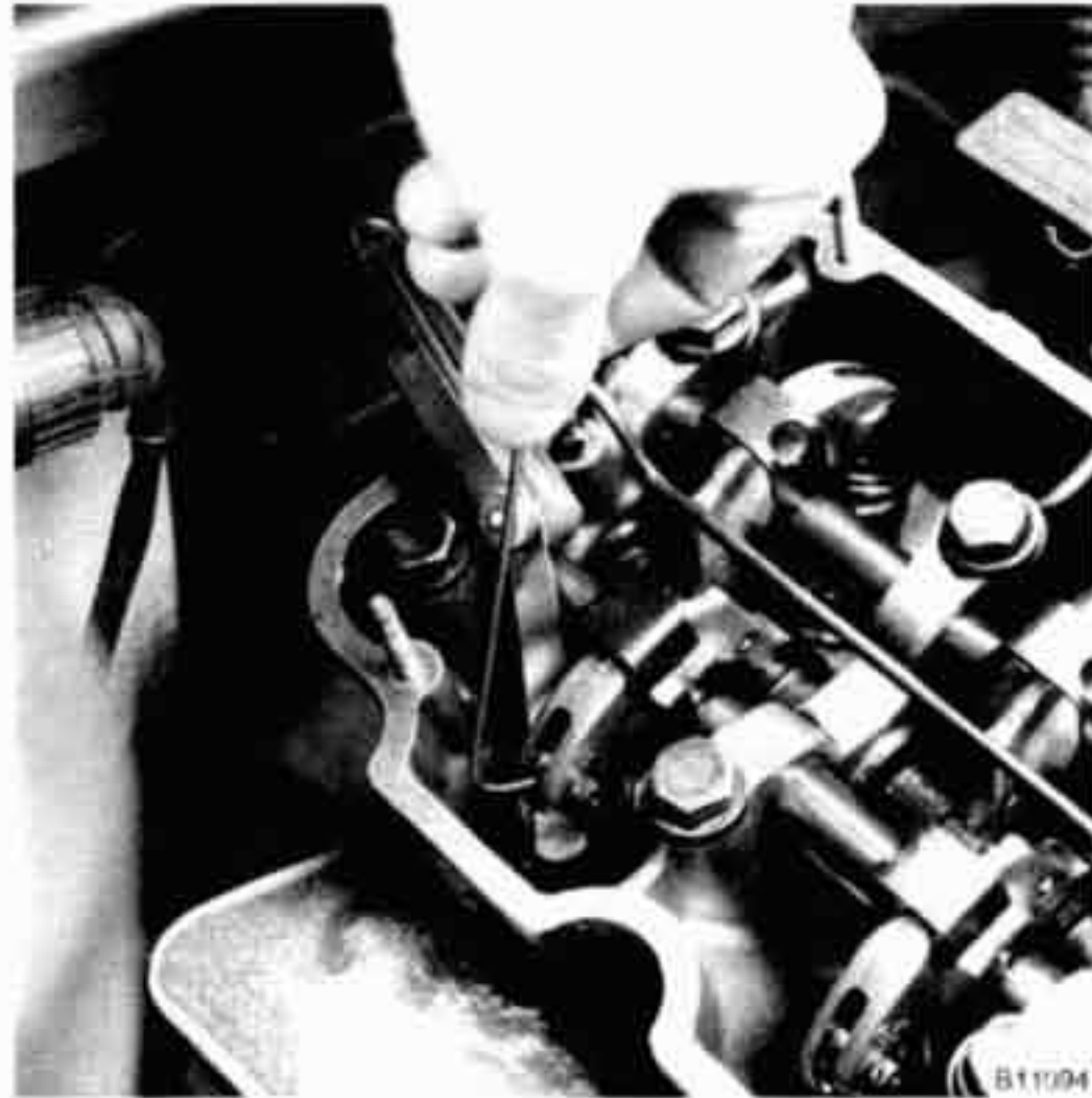
Fig. 16. Valve clearance being adjusted. Stiff wire hook inserted into hole in eccentric.
