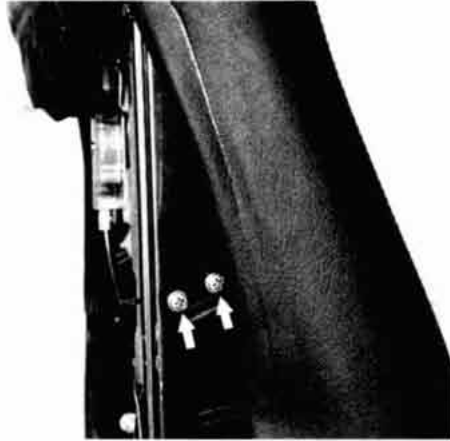
Fig. 13. Headrest adjustment motor screws (arrows).
