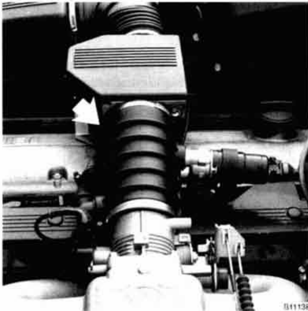
Fig. 22. Intake air boot to be removed (arrow).
