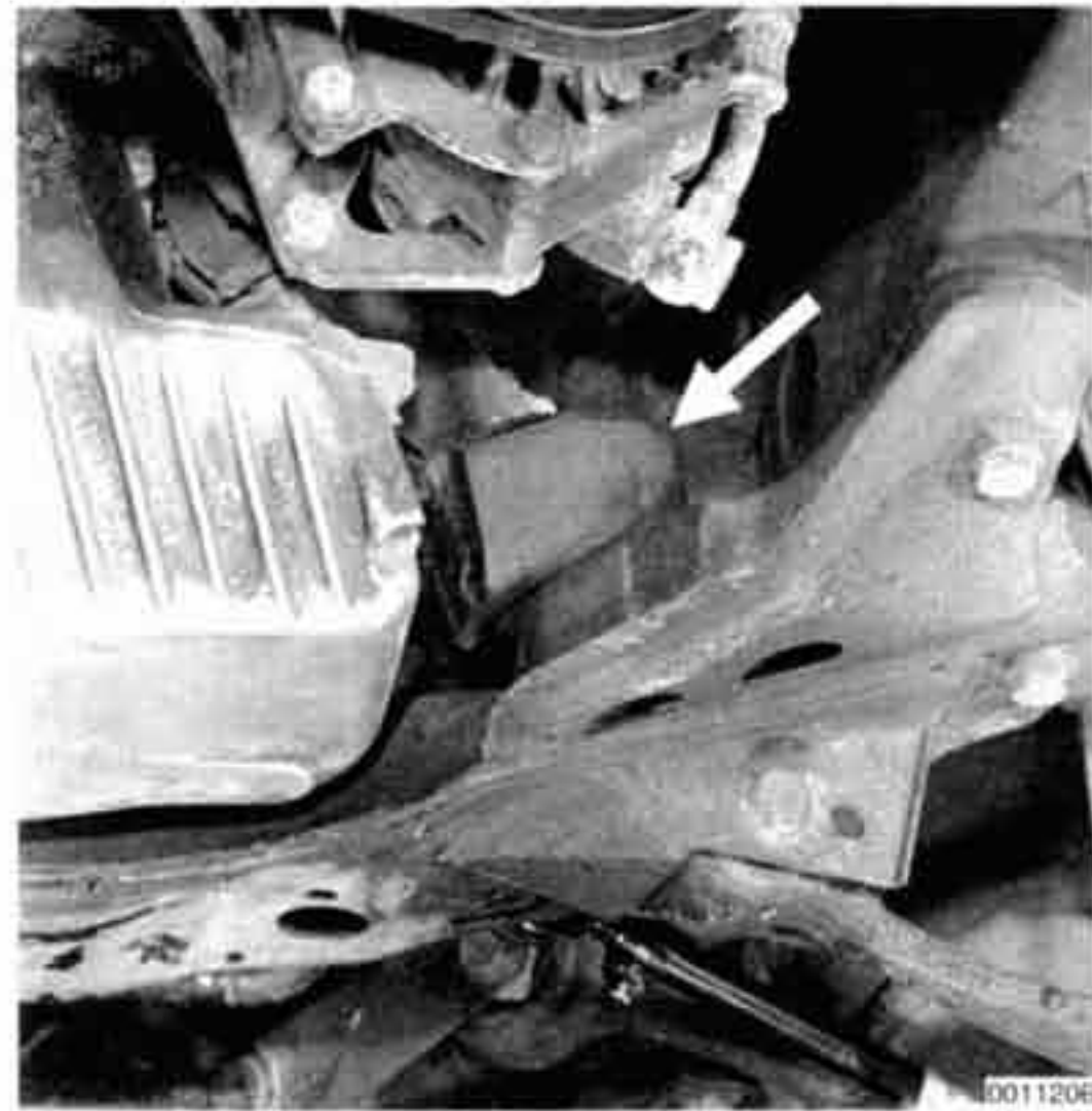
Fig. 17. Left lower engine mount (arrow).
