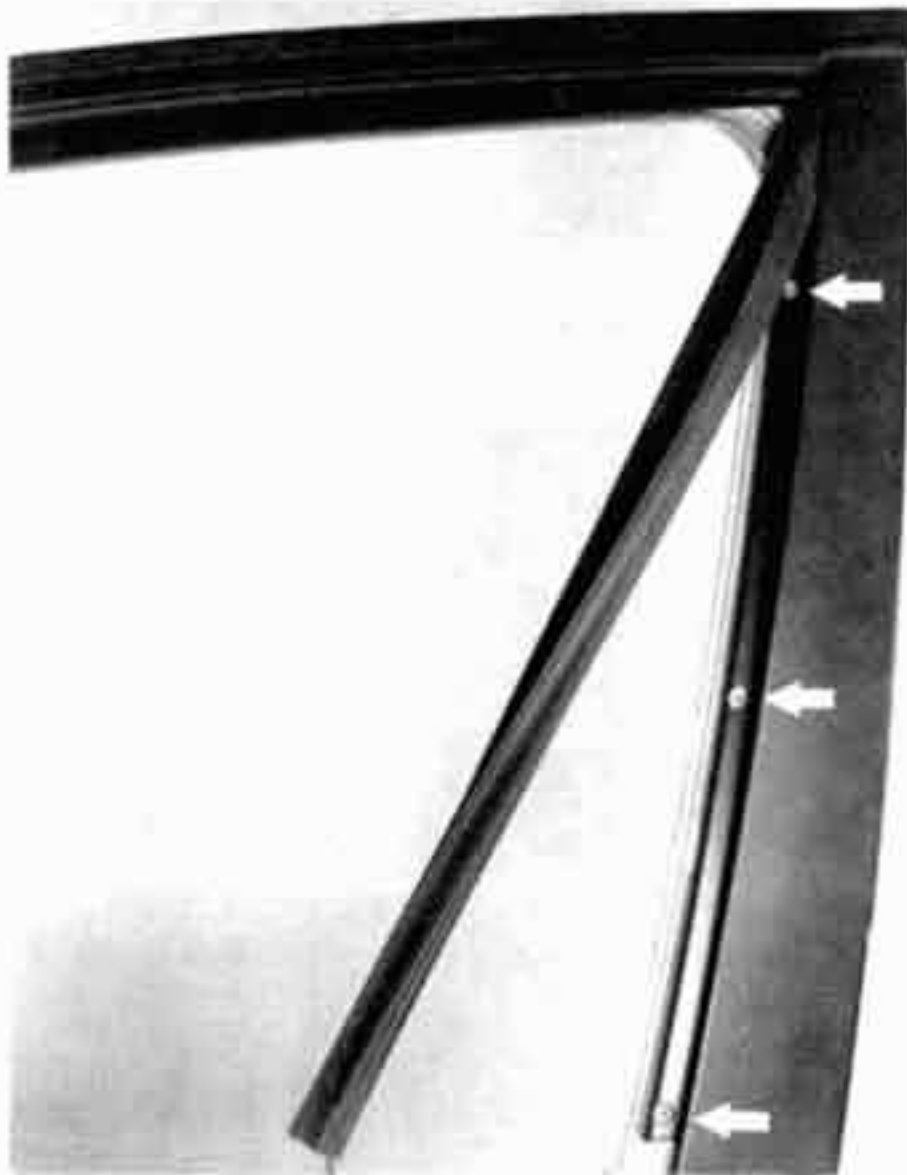
Fig. 4. Remove screws from window trim cover (arrows) and remove cover.
