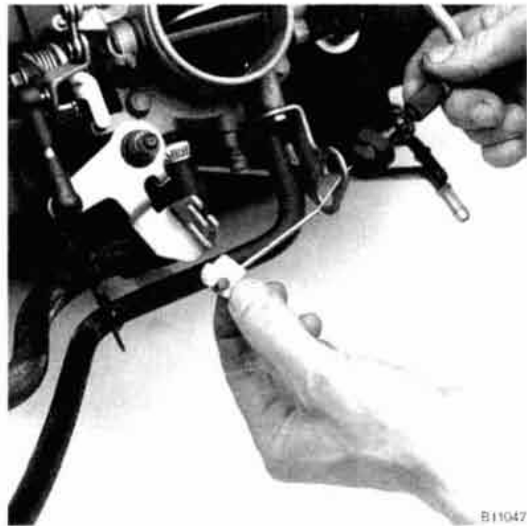
Fig. 8. Throttle cable being removed from throttle lever.
