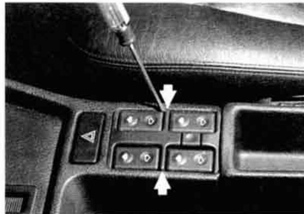
Fig. 7. Window switch being removed from center console. Pry switch alternately at left and right sides (arrows) to remove.
