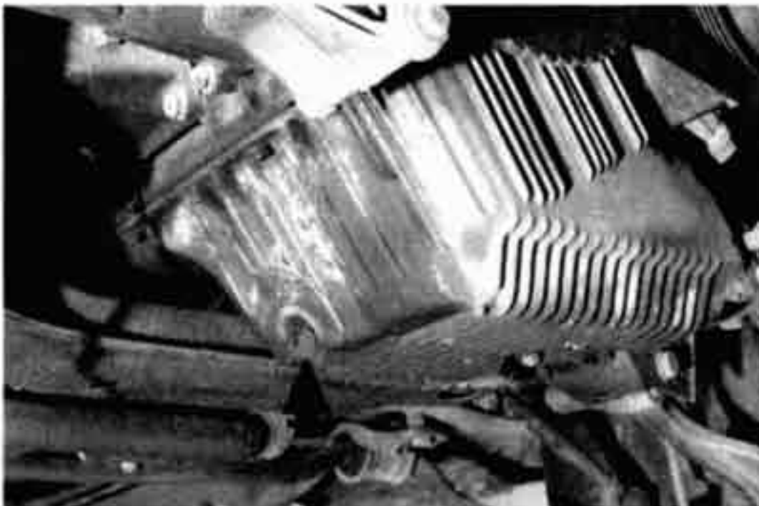
Fig. 3. Engine oil drain plug (arrow) in oil sump.
