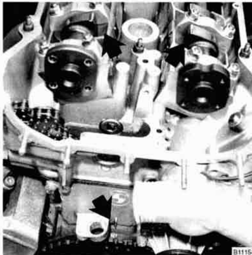
Fig. 38. Engine set to TDC—camshaft lobes face in and 0/T mark (0°TDC) on vibration damper aligns with boss on cover (arrows). Camshaft sprockets shown removed.
