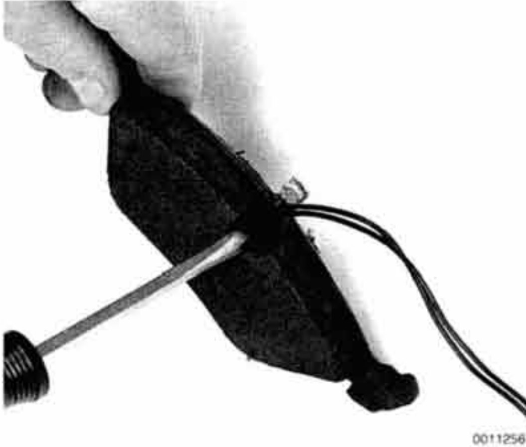
Fig. 5. Brake pad wear sensor being pried from brake pad. If reusing the sensor, use care when removing as they are easily damaged during removal.
