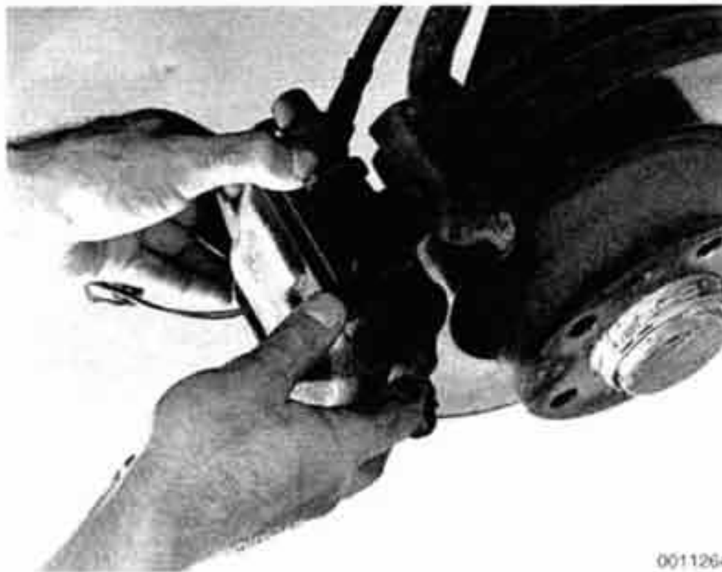
Fig. 4. Front brake caliper being removed.
