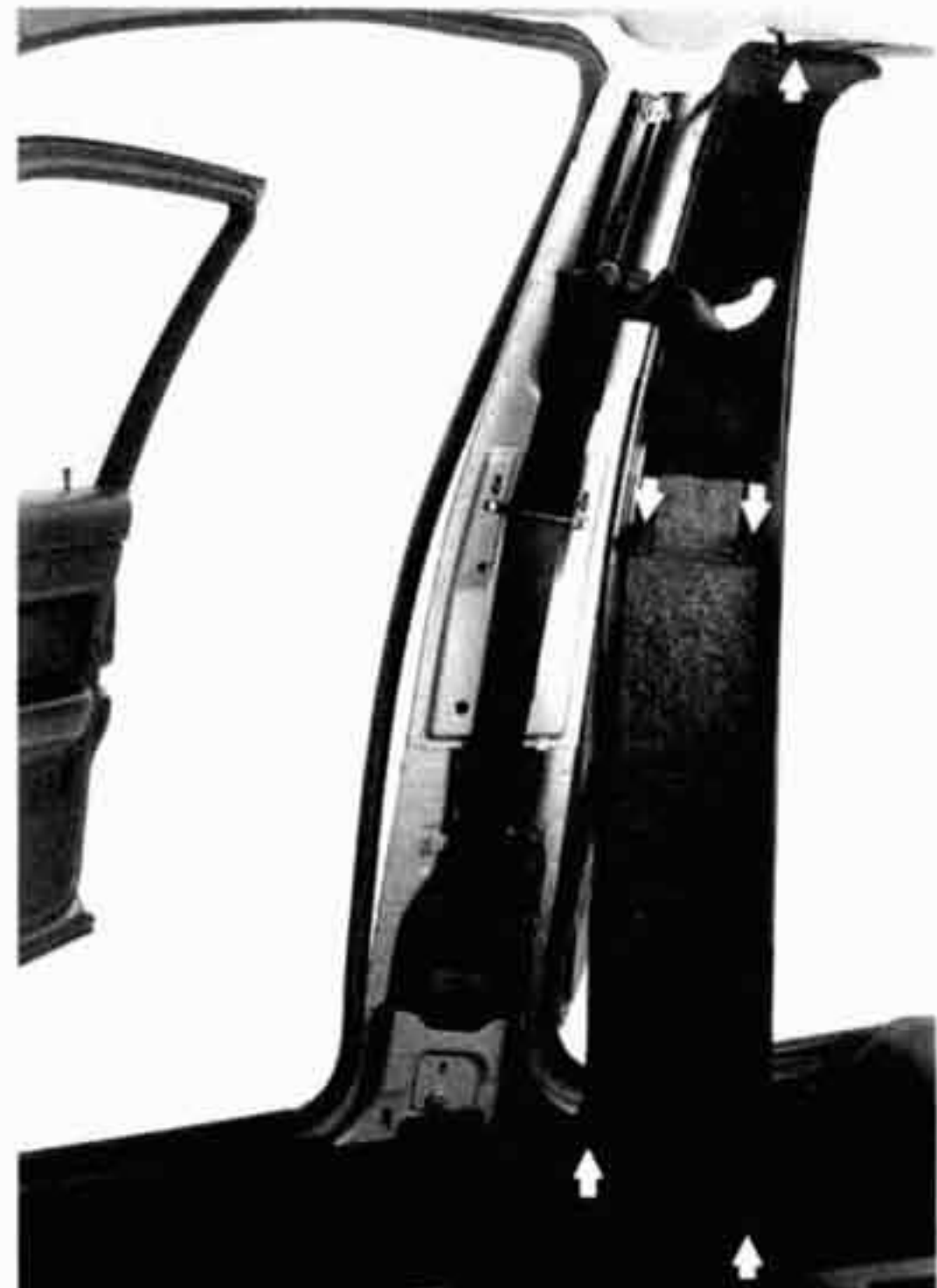
Fig. 1. B-pillar trim panel retaining clips (arrows).
