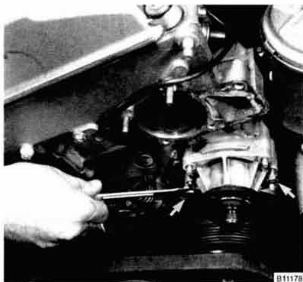
Fig. 13. Coolant pump being removed using two M6 bolts (arrows). Thread bolts in evenly to withdraw pump.
