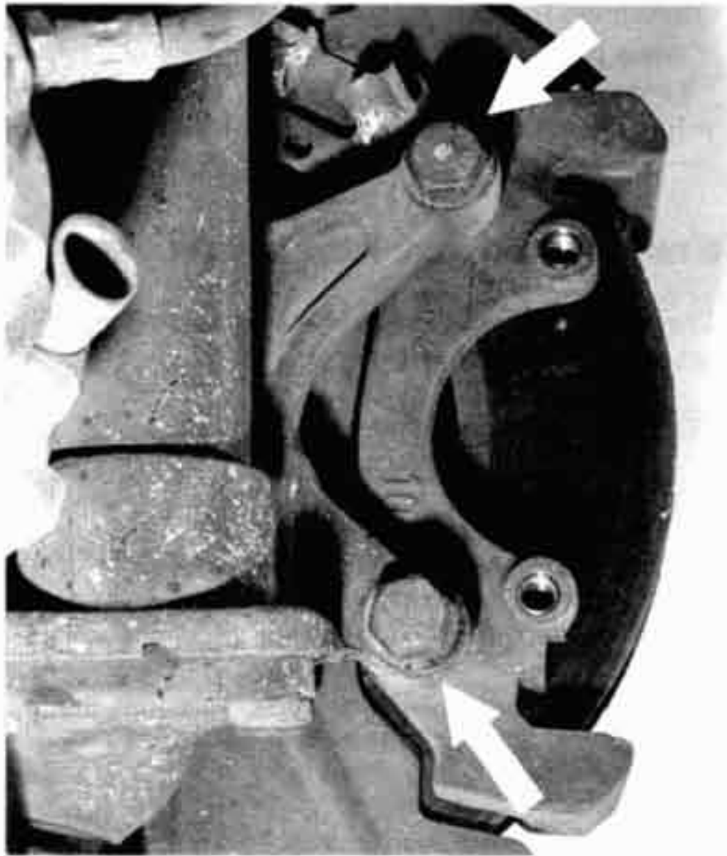
Fig. 8. Front brake pad carrier mounting bolts (arrows). Rear mounting bolts are similar.
