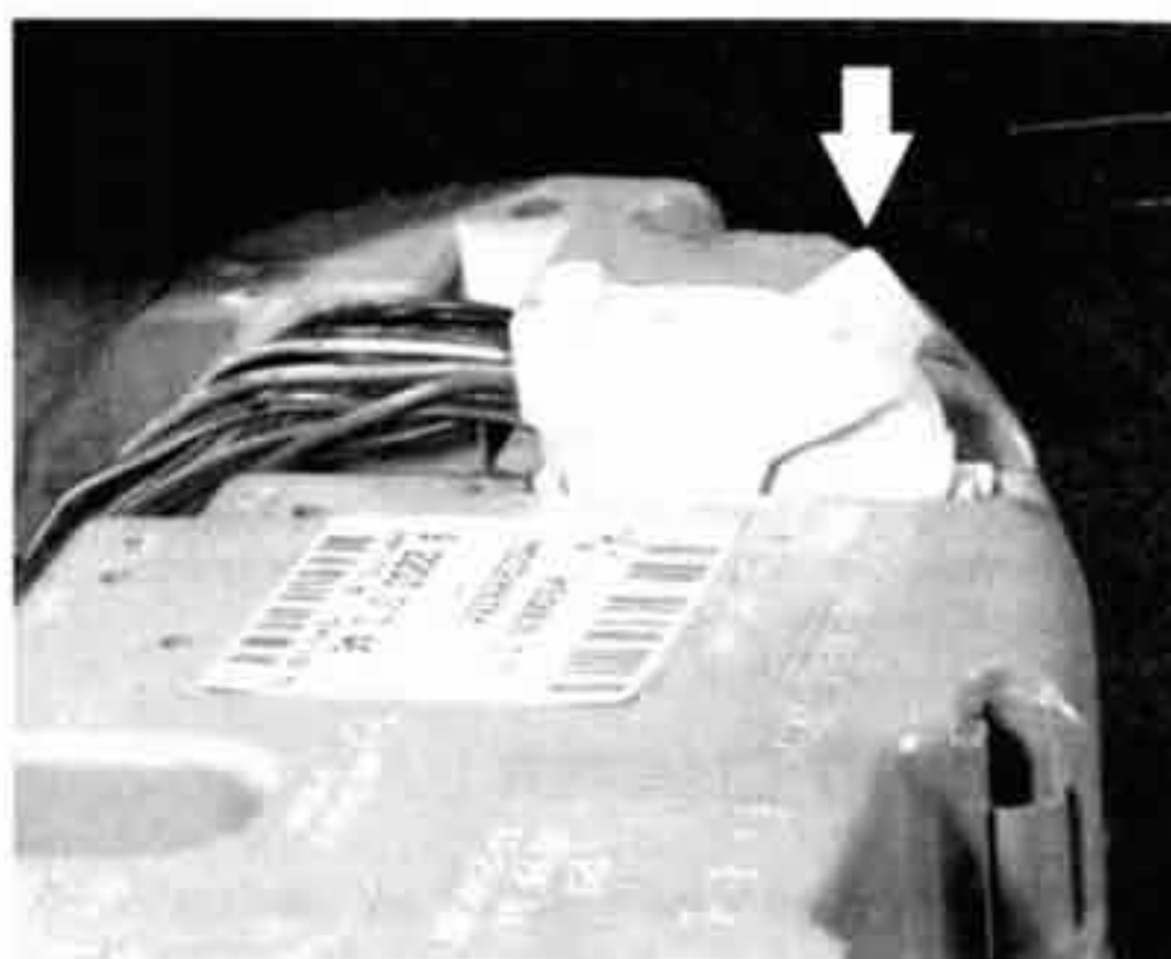
Fig. 2. Pull up on locking lever (arrow) to release instrument cluster connector. Locking lever must be in up position before installing connector.
