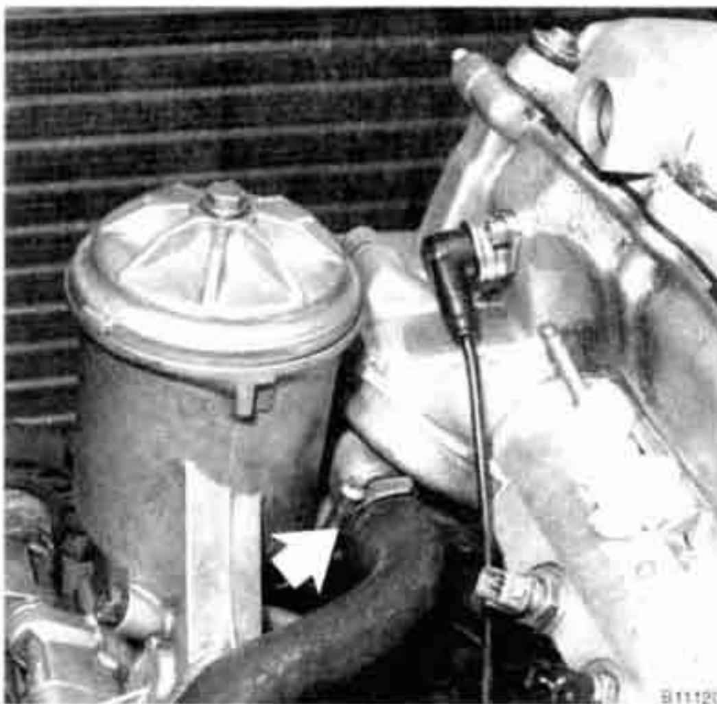
Fig. 6. Coolant hose at oil filter housing (arrow).
