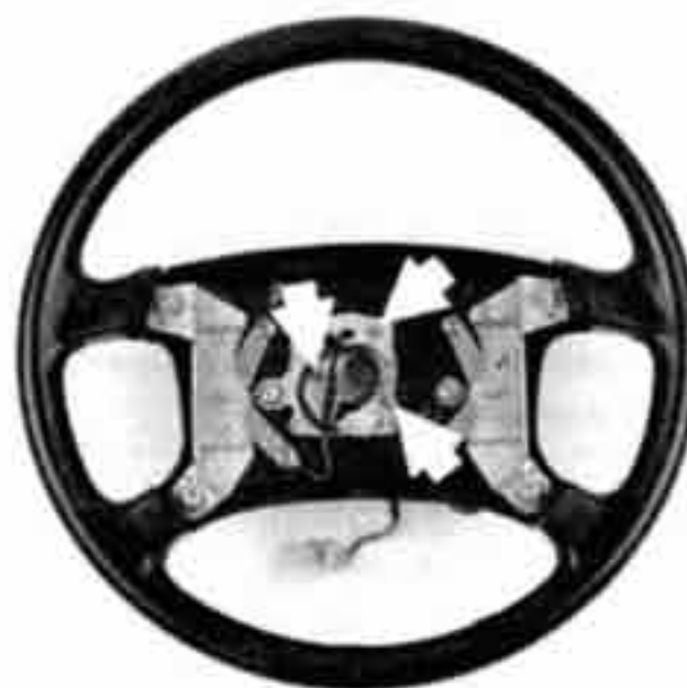
Fig. 9. Airbag contact ring mounting nuts (arrows) on cars with Airbag I. Contact ring used on cars with Airbag II uses screws to mount contact ring.
