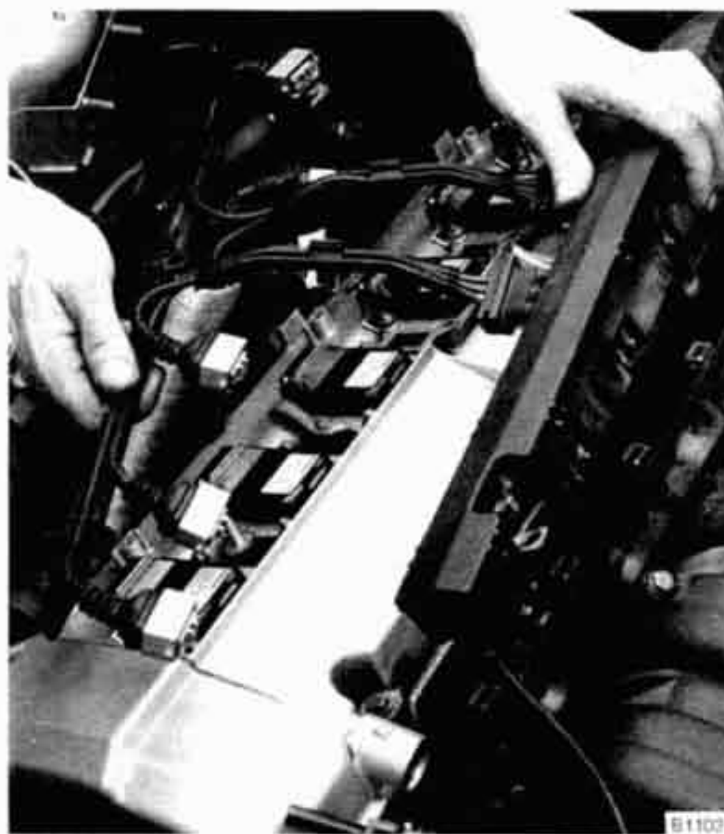
Fig. 15. Remove main harness from top of engine and place at base of windshield.
